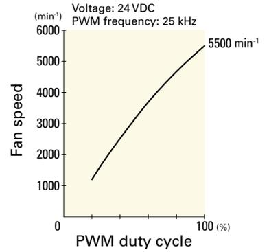
**9WL0824P4H001** With pulse sensor with PWM control function
