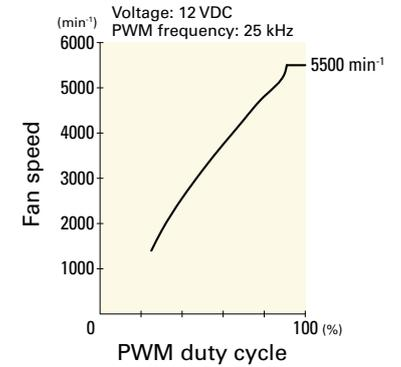
**9WL0812P4H001** With pulse sensor with PWM control function
