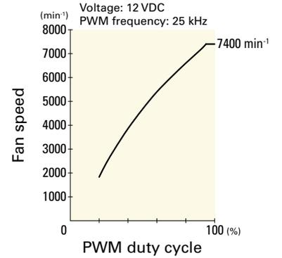
**9WL0812P4G001** With pulse sensor with PWM control function
