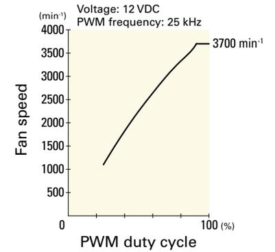
**9WL0824P4J001** With pulse sensor with PWM control function
