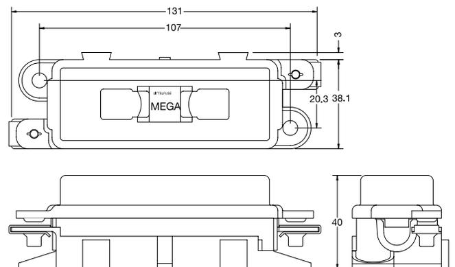
For use with MEGA® fuses the holder offers splash-water-proof protection for use in harsh environments.
