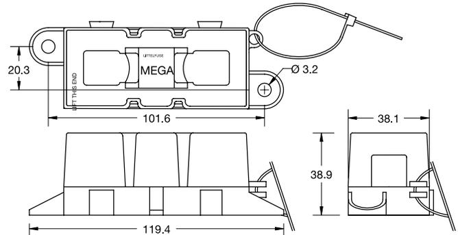
Use with MEGA® fuses up to 500A. Ideal for battery and alternator connections and other heavy gauge cables requiring ultra high current protection. Includes protective cover. Features interconnecting pins on side of fuse block for secure multiple block configurations. Includes M8 threaded studs and hex nuts with lock washers. Fuse not included.
