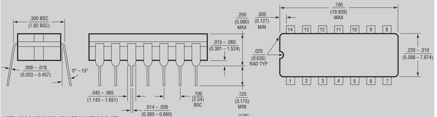
NOTE: LEAD DIMENSIONS APPLY TO SOLDER DIP/PLATE OR TIN PLATE LEADS
