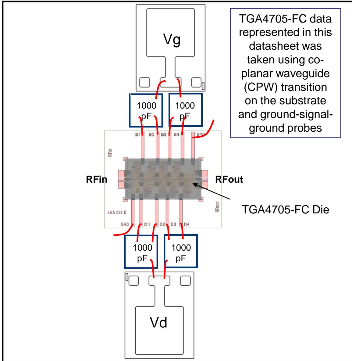
Die is flip-chip soldered to a 15 mil thick alumina test substrate
