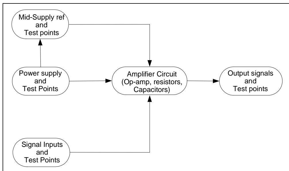
**FIGURE 1-1: MCP6H04 Evaluation Board - Block Diagram.**
