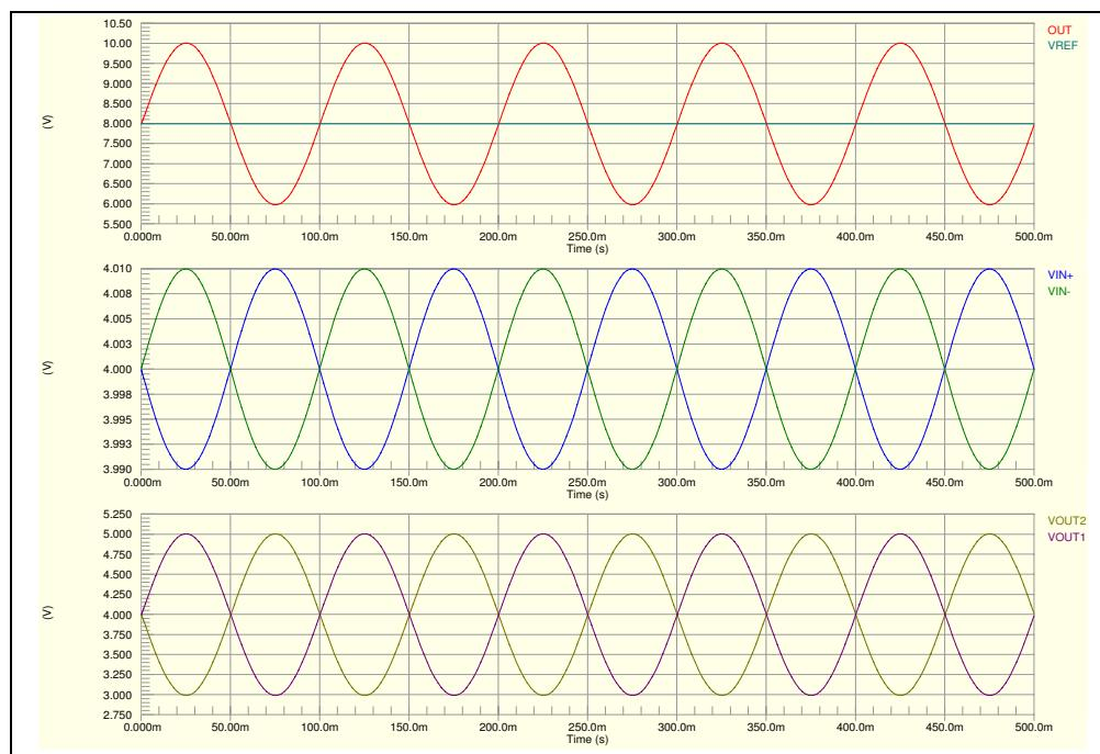
**FIGURE 2-14:** Simulation of the Sine Wave Response.
