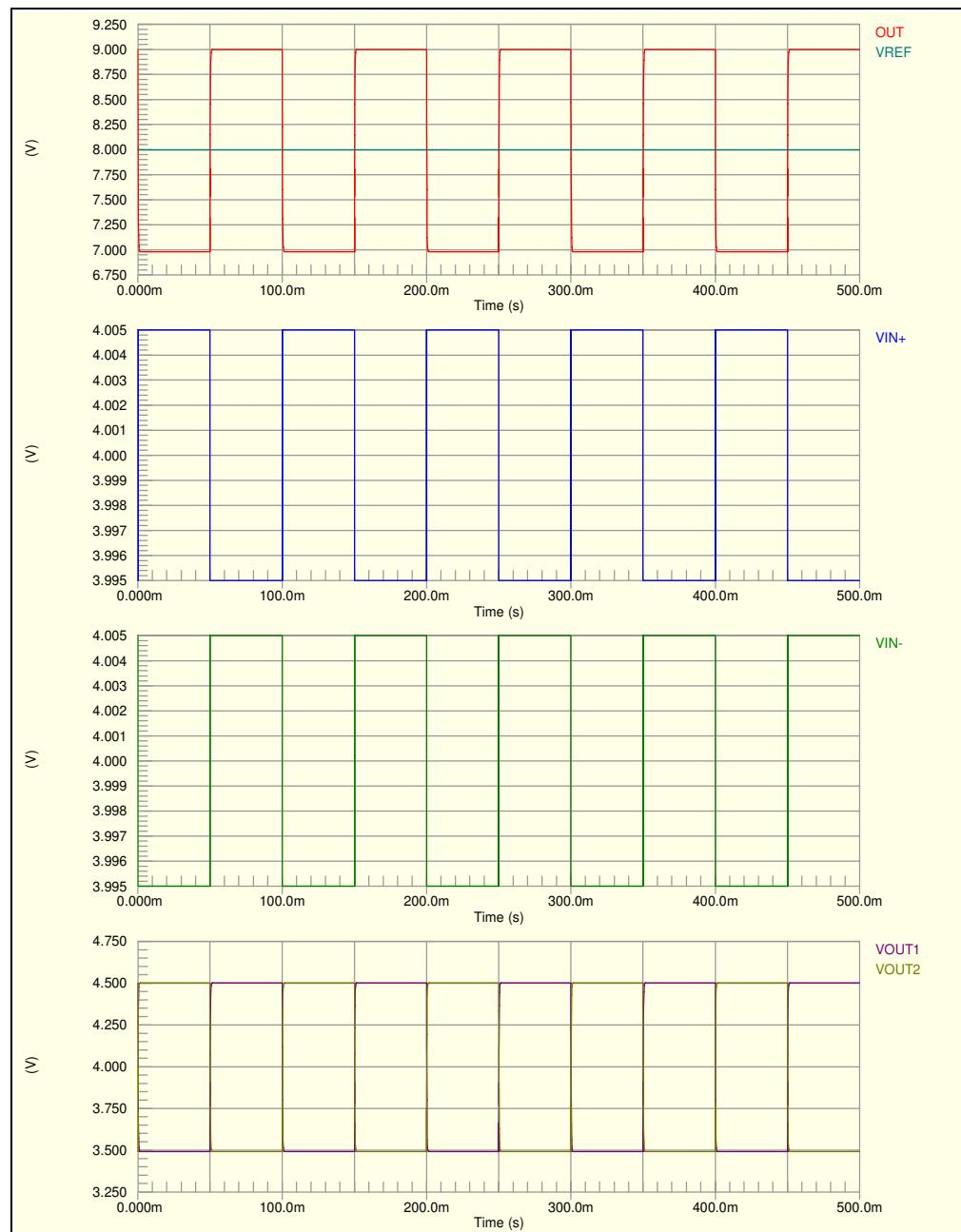
**FIGURE 2-16:** Simulation of the Square Wave Response.
