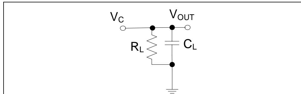
**FIGURE 2-5:** Output Load Block.
