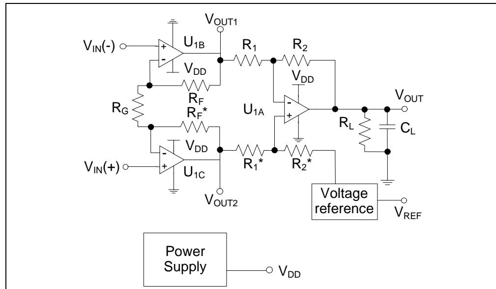
**FIGURE 2-10:** *Instrumentation Amplifier Diagram Block.*
