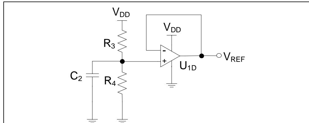
**FIGURE 2-4:** Mid-Supply Reference Block.
