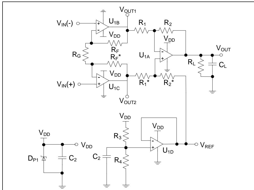
**FIGURE 2-1:** MCP6H04 Evaluation Board Circuit Diagram.
