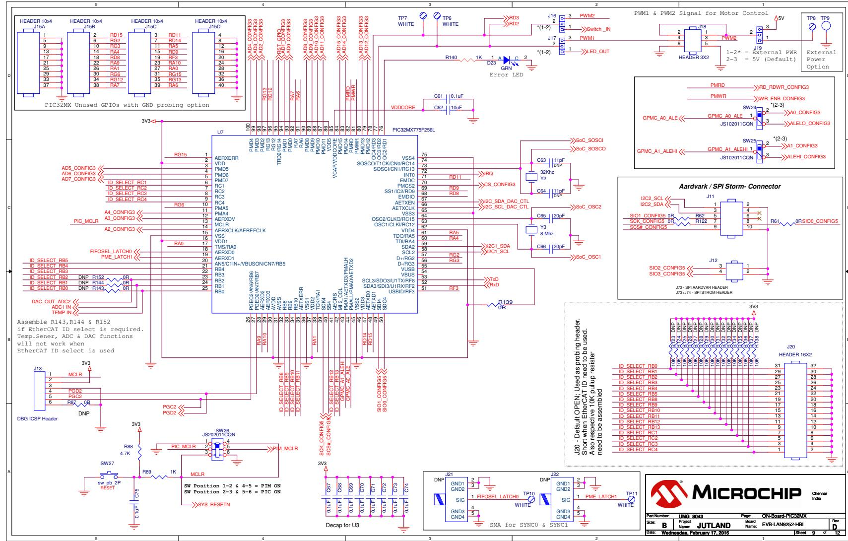
FIGURE B-8: EVB-LAN9252-HBI+ SCHEMATIC GPIOs
