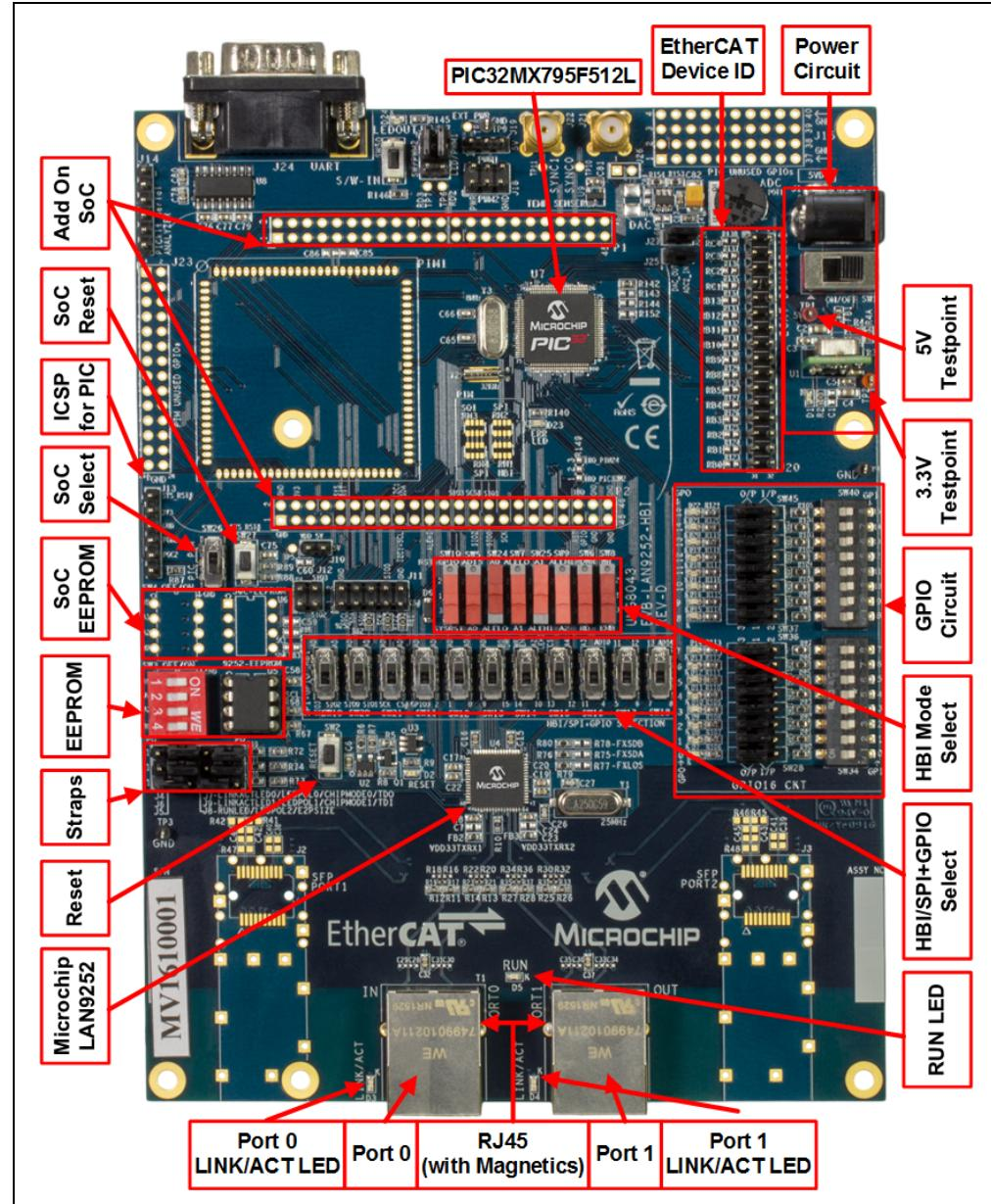
**FIGURE 2-2: EVB-LAN9252-HBI+ TOP VIEW NEW FEATURE CALLOUTS**
