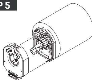
1. Fasten the Base on the motor (Tool C may need to be rotated to allow for some mounting configurations).
