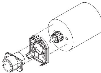
1. Insert Tool A as a spacer that defines the distance to the mounting surface.
