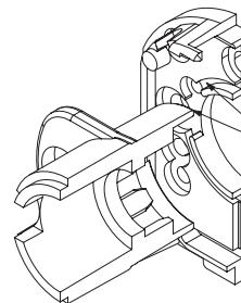
Align Tool C with flange on Base
