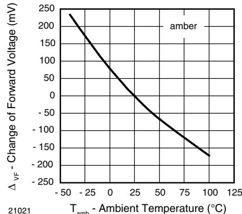
Figure 10. Change of Forward Voltage vs. Ambient Temperature
