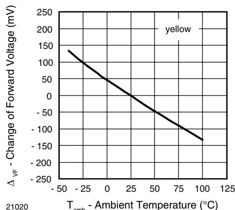
Figure 9. Change of Forward Voltage vs. Ambient Temperature
