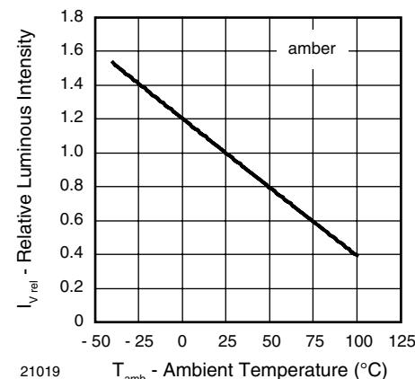
Figure 8. Relative Lum. Intensity vs. Ambient Temperature
