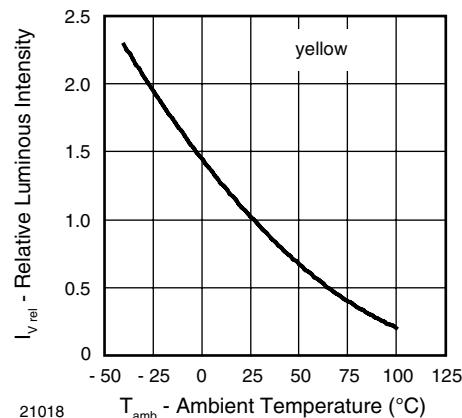
Figure 7. Relative Lum. Intensity vs. Ambient Temperature
