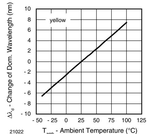
Figure 11. Change of Dominant Wavelength vs. Ambient Temperature
