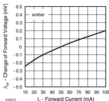
Figure 6. Change of Forward Voltage vs. Forward Current
