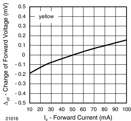
Figure 5. Change of Forward Voltage vs. Forward Current
