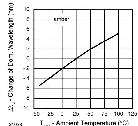
Figure 12. Change of Dominant Wavelength vs. Ambient Temperature
