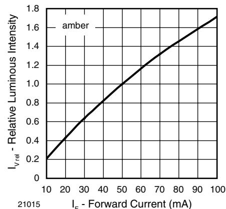
Figure 4. Relative Luminous Intensity vs. Forward Current
