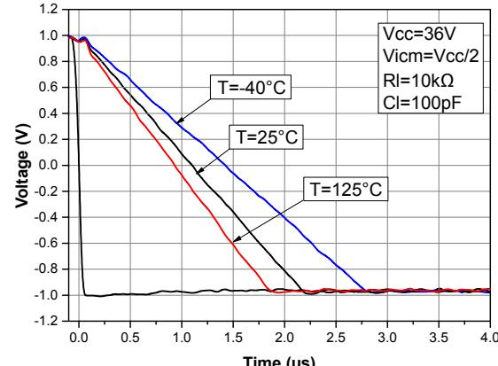
**Figure 19. Positive slew rate at  $V_{CC} = 36$  V**
