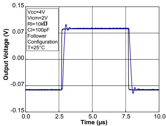
**Figure 28. Output desaturation vs. time**
