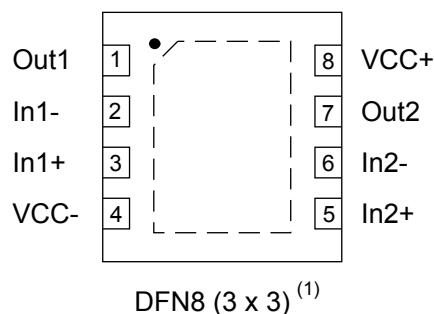
1. Exposed pad can be left floating or connected to ground.
