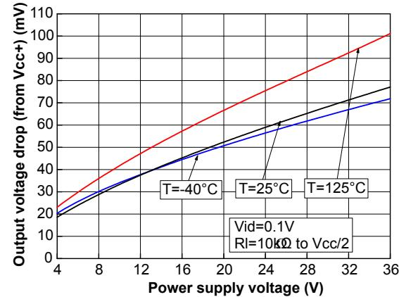
**Figure 17. Output voltage ( $V_{ol}$ ) vs. supply voltage**
