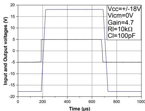
**Figure 29. Amplifier behavior close to the rails at  $V_{CC} = 36\text{ V}$**
