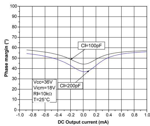
**Figure 25. Phase margin vs. capacitive load**
