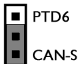
Figure 8-4: Can Operation Mode Selection (J6)
