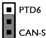
Figure 8-4: Can Operation Mode Selection (J6)
