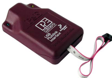
Figure 10-1: P&E's USB Multilink (USB-ML-12 shown)
