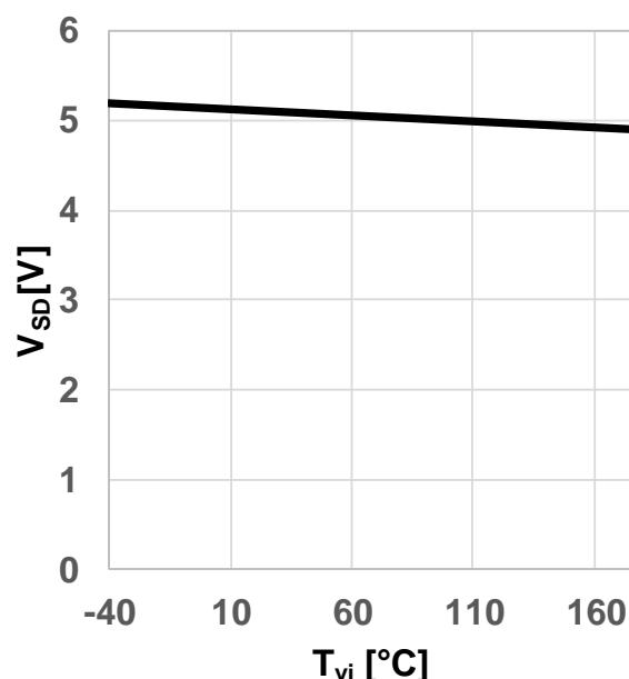
**Figure 12** Typical body diode forward voltage as function of junction temperature
