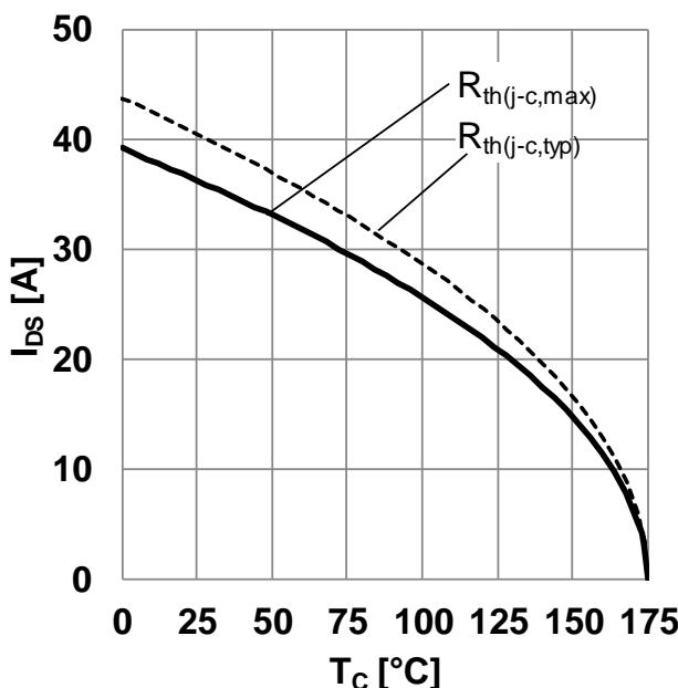
**Figure 3 Maximum DC drain to source current as a function of case temperature limited by bond wire**
