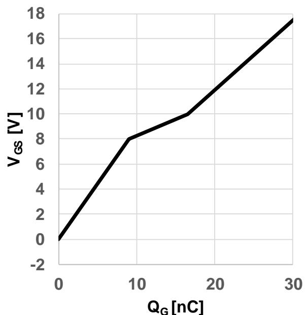
**Figure 10** Typical gate charge
