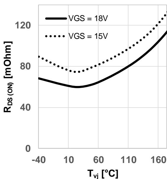
**Figure 9** Typical on-resistance as a function of junction temperature
