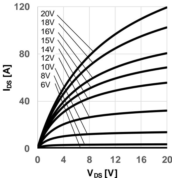
**Figure 7** Typical output characteristic,  $V_{GS}$  as parameter
