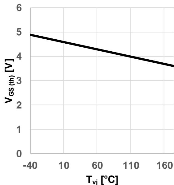
**Figure 6** Typical gate-source threshold voltage as a function of junction temperature
