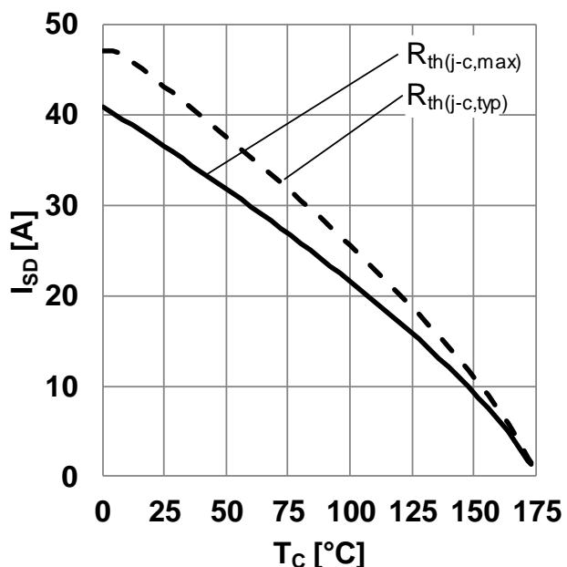
**Figure 4 Maximum source to drain current as a function of case temperature limited by bond wire**
