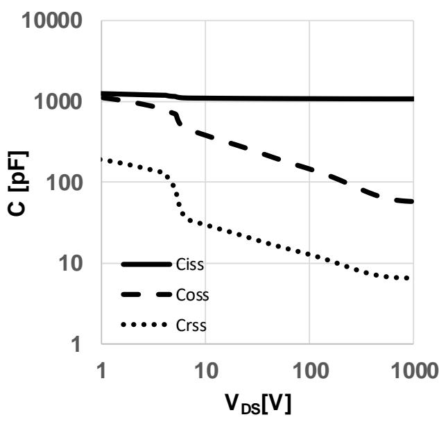
**Figure 11** Typical capacitance as a function of drain-source voltage
