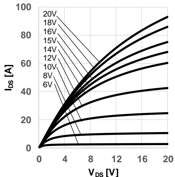
**Figure 8** Typical output characteristic,  $V_{GS}$  as parameter
