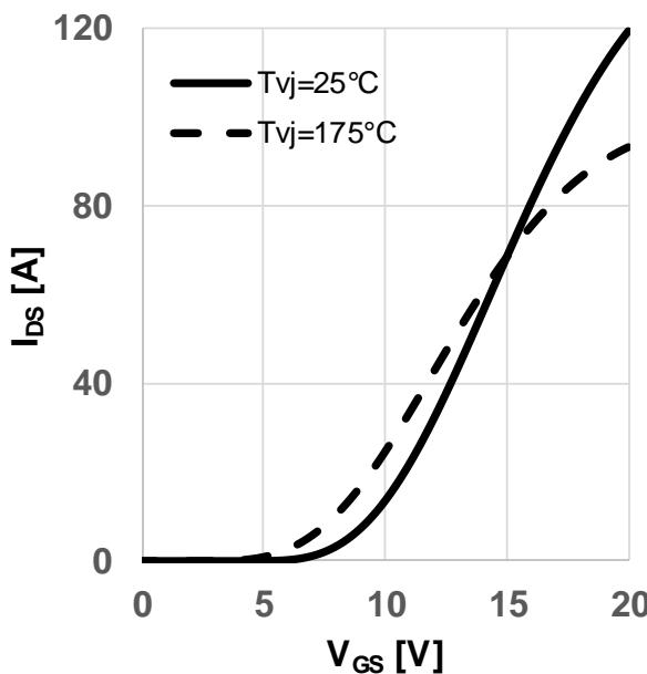
**Figure 5** Typical transfer characteristic
