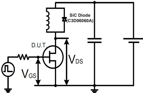
**Figure 15. Switching Time Test Circuit**
