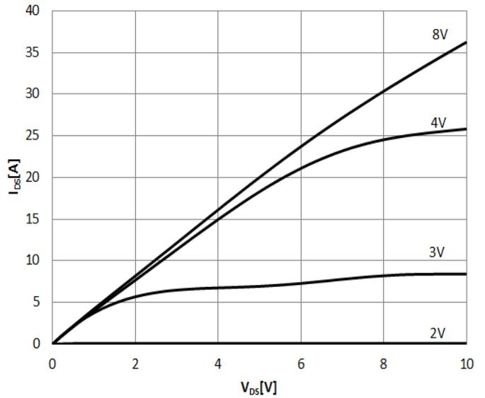
**Figure 2. Typical Output Characteristics  $T_J=150^\circ\text{C}$**
