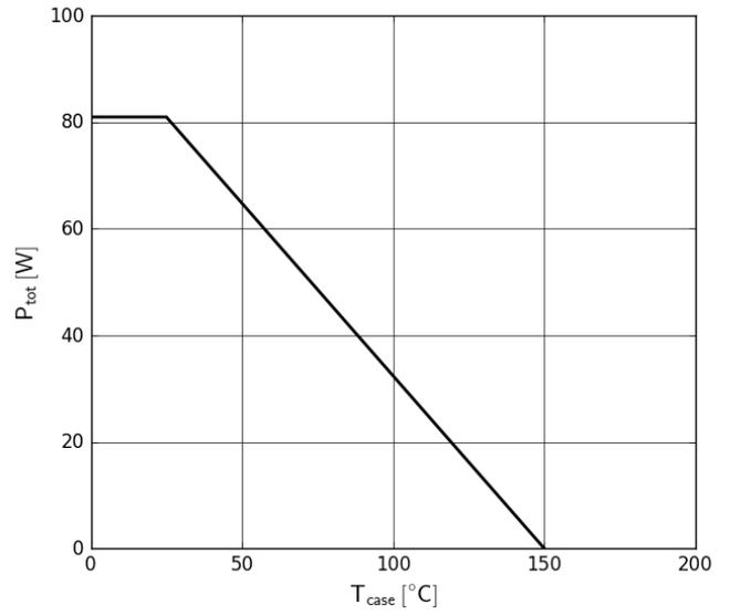
Figure 14. Power Dissipation
