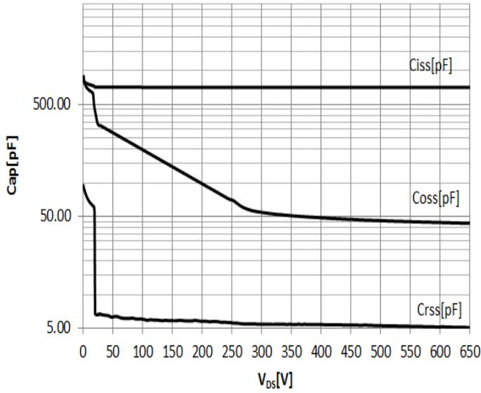
Figure 5. Typical Capacitance
