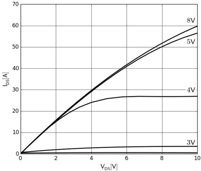
**Figure 1. Typical Output Characteristics  $T_J=25^\circ\text{C}$**
