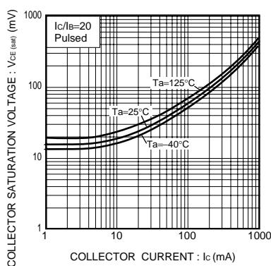
Fig.4 Collector-emitter saturation voltage vs. collector current ( II )
