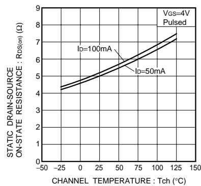
Fig.15 Static drain-source on-state resistance vs. channel temperature
