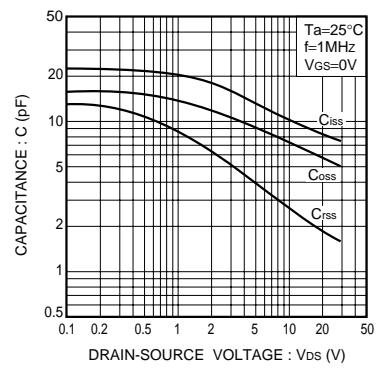
Fig.19 Typical capacitance vs.
