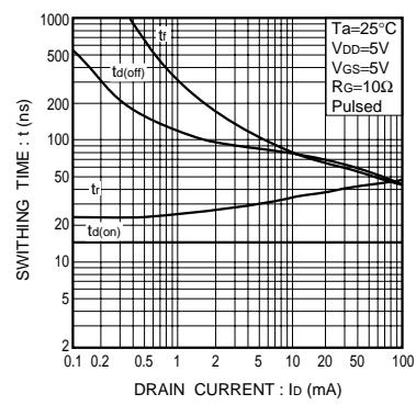
Fig.20 Switching characteristics
