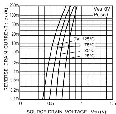
Fig.17 Reverse drain current vs. source-drain voltage ( I )
