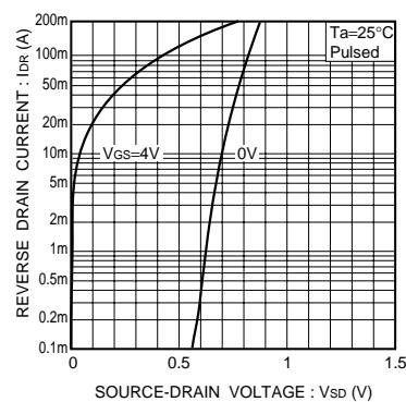
Fig.18 Reverse drain current vs.
