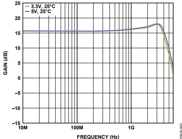
Figure 3. Gain vs. Frequency Response for  $200 \Omega$  Differential Load,  $V_{POS} = 3.3$  V and  $V_{POS} = 5$  V,  $25^\circ\text{C}$
