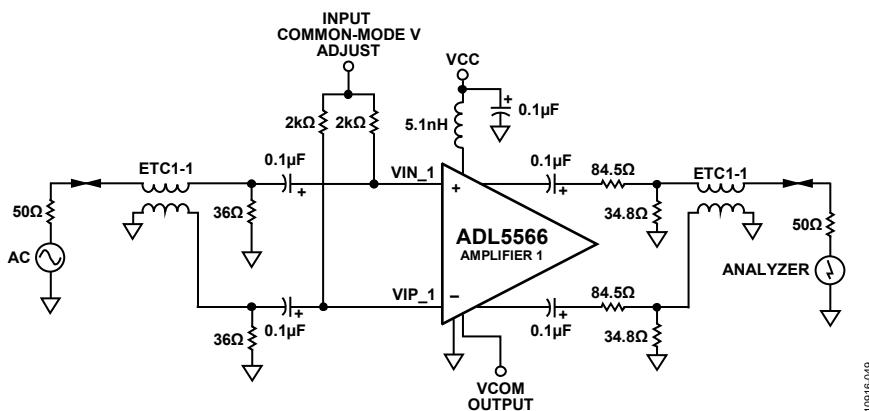
Figure 51. Distortion Measurement Circuit for Various Common-Mode Voltages
