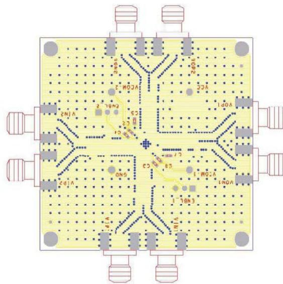
*Figure 55. Layout of Evaluation Board, Circuit Side*
