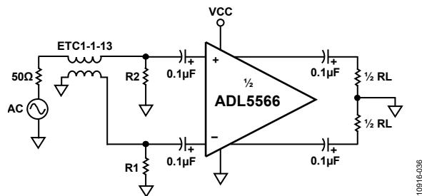
Figure 37. Differential Input to Differential Output Configuration
