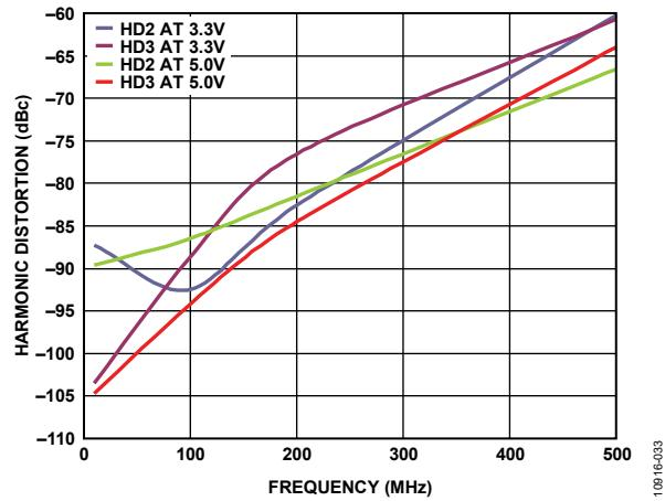
Figure 24. Single-Ended Harmonic Distortion (HD2/HD3) vs. Frequency,  $V_{POS} = 3.3$  V and  $V_{POS} = 5$  V,  $V_{OUT} = 2$  Vp-p,  $R_L = 200 \Omega$
