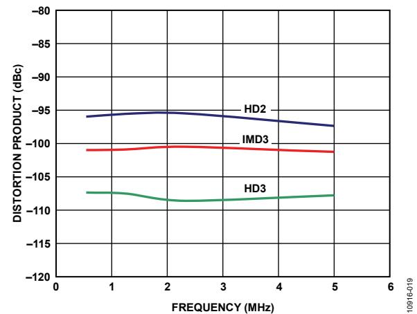
Figure 25. Low Frequency Distortion (HD2/HD3/IMD3) vs. Frequency, Output Level at 2 Vp-p,  $R_L = 200 \Omega$ ,  $V_{POS} = 3.3$  V
