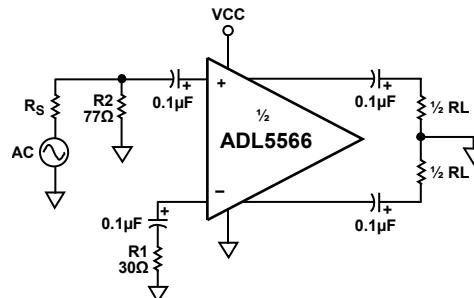
Figure 39. Single-Ended Input to Differential Output Configuration
