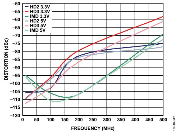
Figure 43. IMD, HD2, and HD3 vs. Frequency,  $A_V = 6$  dB, 2 Vp-p Output,  $V_{POS} = 3.3$  and  $V_{NEG} = 5$  V
