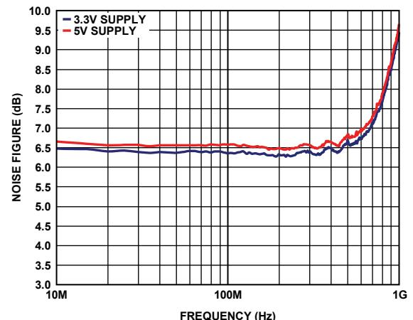
Figure 8. Noise Figure vs. Frequency at  $V_{POS} = 3.3$  V,  $V_{POS} = 5$  V,  $25^\circ\text{C}$
