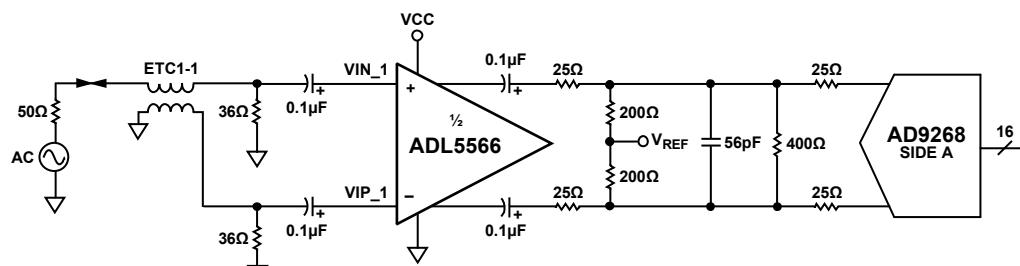
Figure 47. Wideband ADC Interfacing Example Featuring the AD9268
