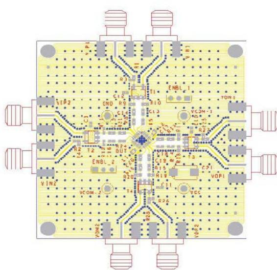
*Figure 54. Layout of Evaluation Board, Component Side*
