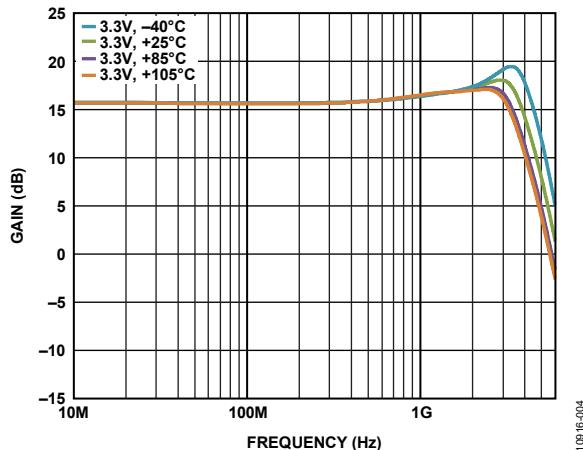
Figure 4. Gain vs. Frequency Response for  $200 \Omega$  Differential Load, Four Temperatures,  $V_{POS} = 3.3$  V
