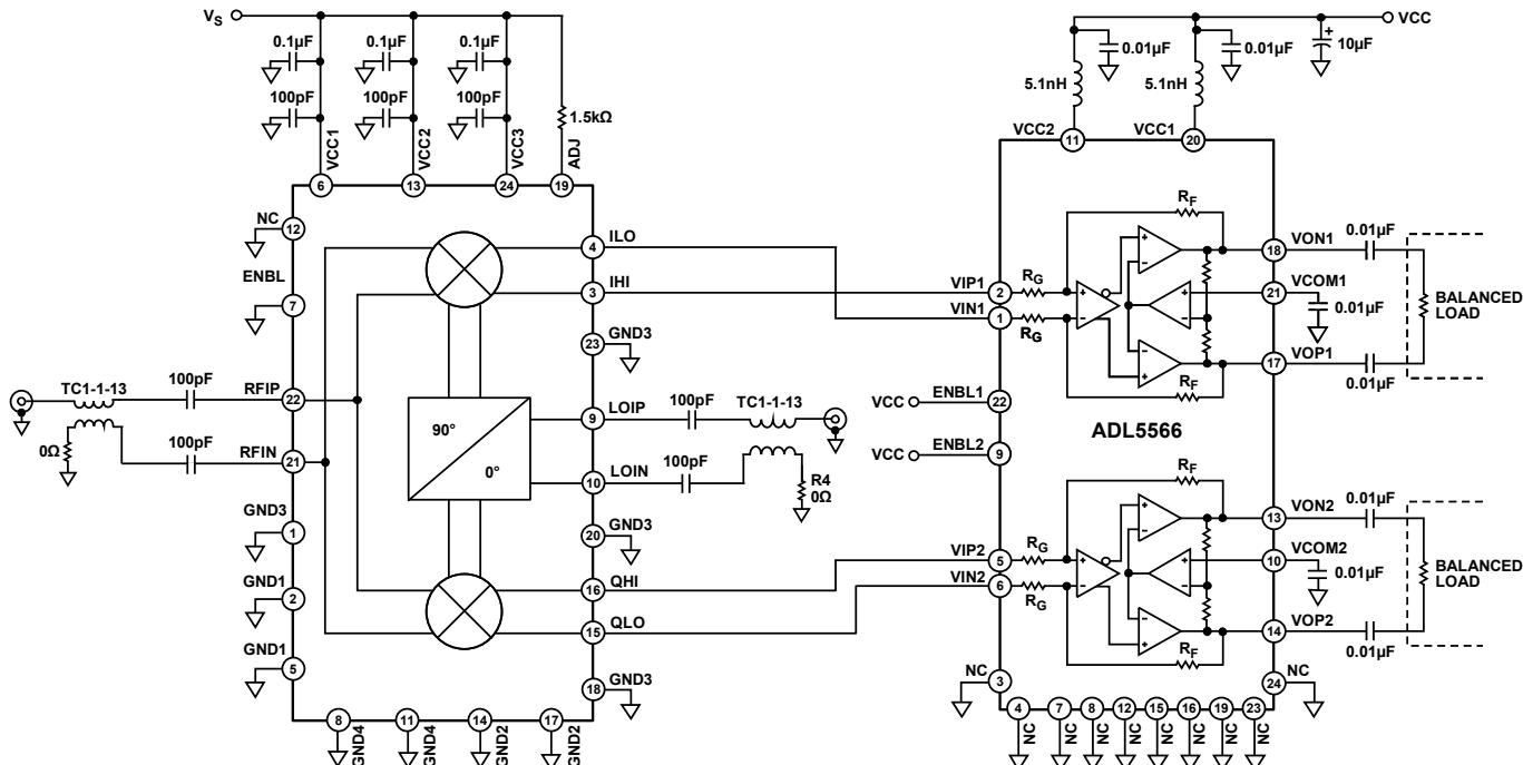
Figure 48. DC-Coupled Interface Example Featuring the ADL5380
