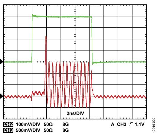
Figure 26. ENBLx Time Domain Response,  $V_{POS} = 3.3$  V
