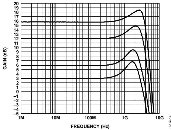
Figure 42. SDD21,  $V_{POS} = 3.3$  V, Three Gains, 25°C
