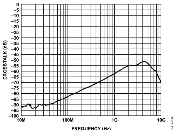
Figure 33. Output Referred Crosstalk, Channel A to Channel B,  $V_{POS} = 3.3\text{ V}$ ,
