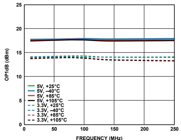
Figure 7. OP1dB vs. Frequency for  $200 \Omega$  Differential Load, Four Temperatures,  $V_{POS} = 3.3$  V,  $V_{POS} = 5$  V
