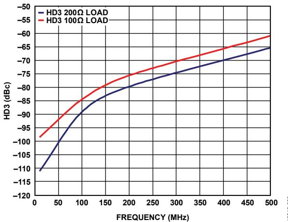
Figure 23. HD3 vs. Frequency,  $R_L = 100 \Omega$  and  $R_L = 200 \Omega$ ,  $V_{POS} = 3.3$  V, Input Common-Mode = 1.65 V, Output Common-Mode = 1.25 V,  $V_{OUT} = 1.5$  Vp-p
