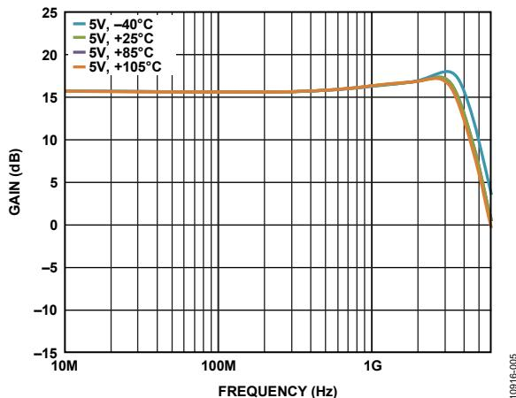
Figure 5. Gain vs. Frequency Response for  $200 \Omega$  Differential Load, Four Temperatures,  $V_{POS} = 5$  V
