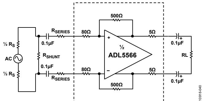
Figure 41. Gain Adjustment Using a Series Resistor Show
