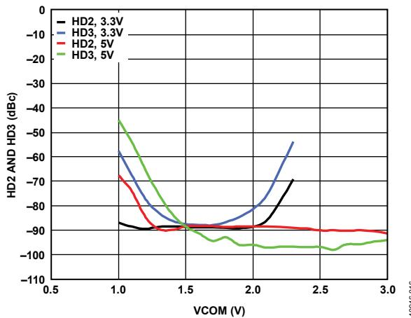
Figure 21. Harmonic Distortion (HD2/HD3) vs. VCOM, Output Level at 2 Vp-p,  $R_L = 200 \Omega$ ,  $V_{POS} = 3.3$  V and  $V_{POS} = 5$  V, Frequency = 100 MHz
