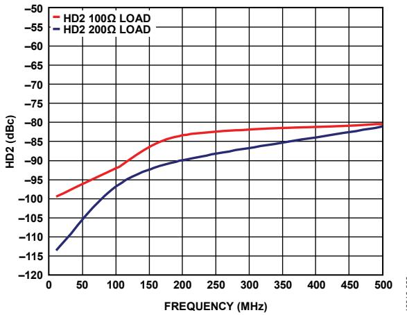
Figure 22. HD2 vs. Frequency,  $R_L = 100 \Omega$  and  $R_L = 200 \Omega$ ,  $V_{POS} = 3.3$  V, Input Common-Mode = 1.65 V, Output Common-Mode = 1.25 V,  $V_{OUT} = 1.5$  Vp-p
