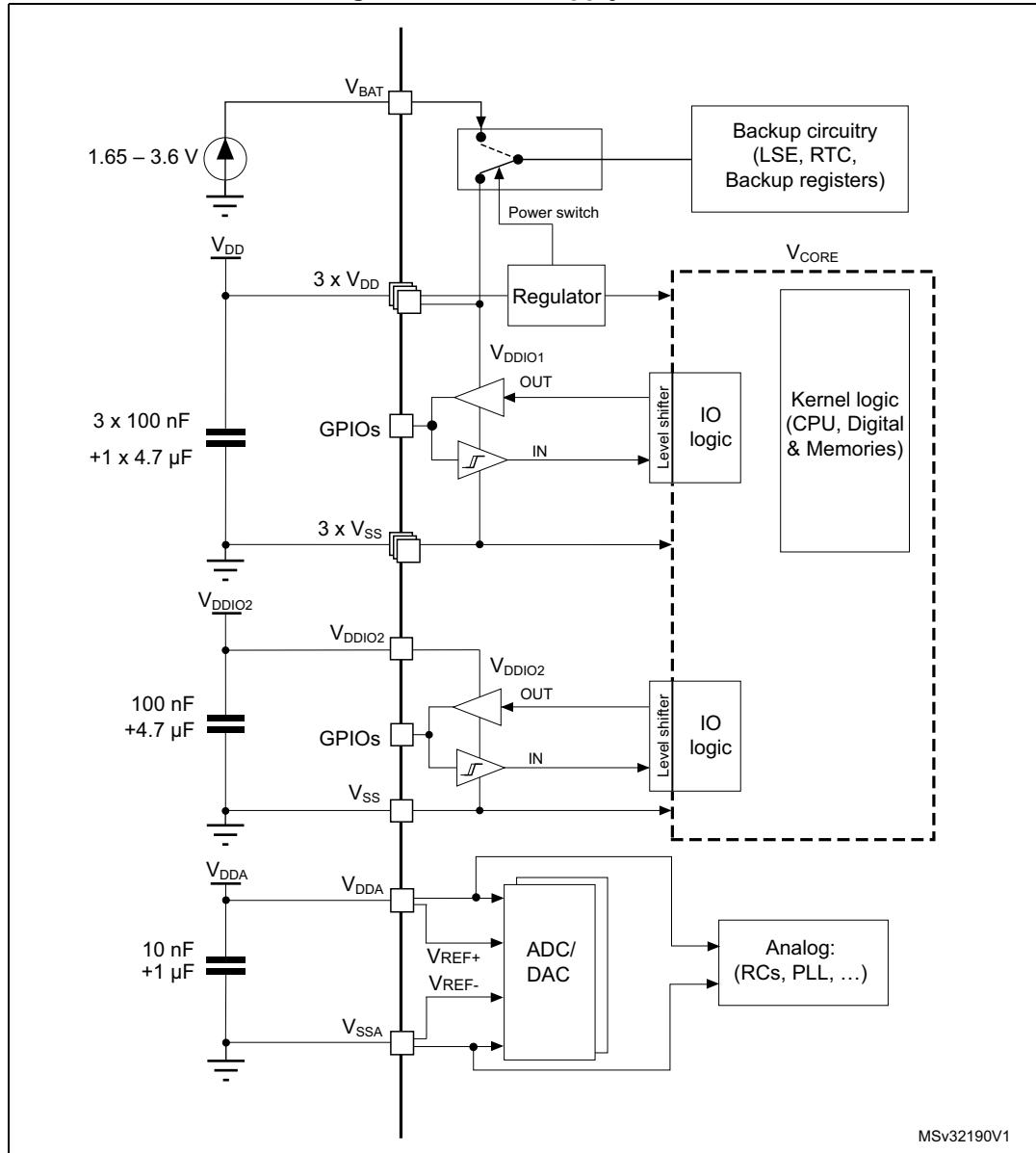
**Caution:** Each power supply pair ( $V_{DD}/V_{SS}$ ,  $V_{DDA}/V_{SSA}$  etc.) must be decoupled with filtering ceramic capacitors as shown above. These capacitors must be placed as close as possible to, or below, the appropriate pins on the underside of the PCB to ensure the good functionality of the device.
