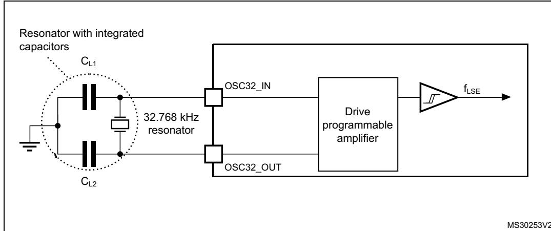
Note: An external resistor is not required between OSC32\_IN and OSC32\_OUT and it is forbidden to add one.
