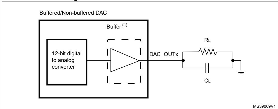
1. The DAC integrates an output buffer that can be used to reduce the output impedance and to drive external loads directly without the use of an external operational amplifier. The buffer can be bypassed by configuring the BOFFx bit in the DAC\_CR register.
