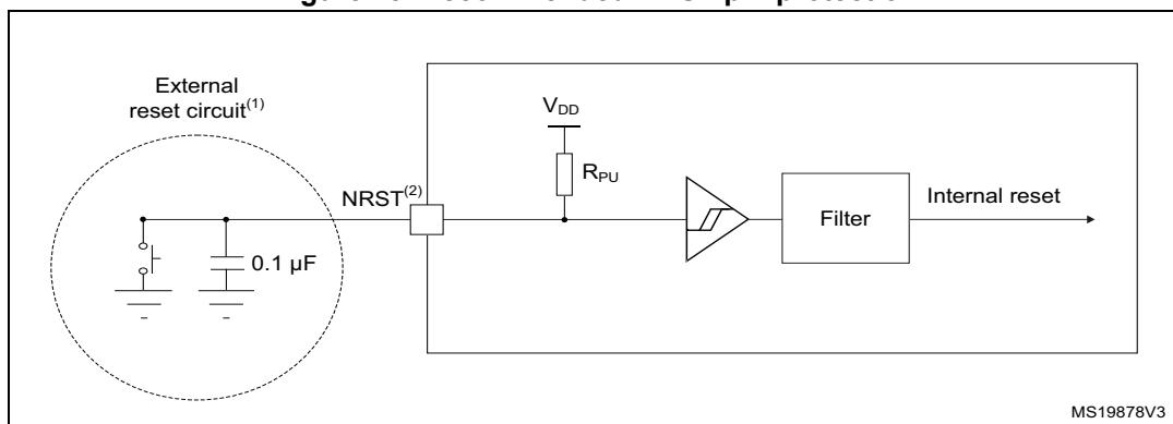
1. The external capacitor protects the device against parasitic resets.
