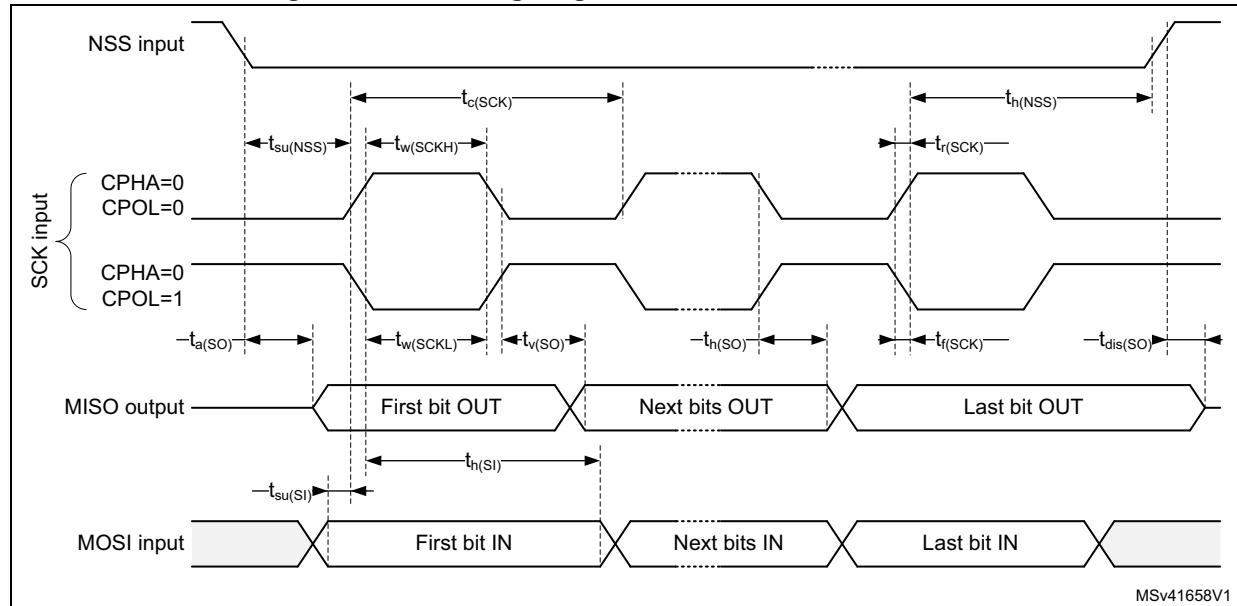
Figure 31. SPI timing diagram - slave mode and CPHA = 1
