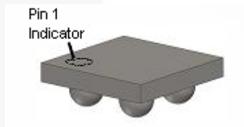
Figure 3. 1 x 1 mm WLCSP Bumps Facing Down
