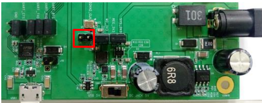
Figure 7: Pin header J1
