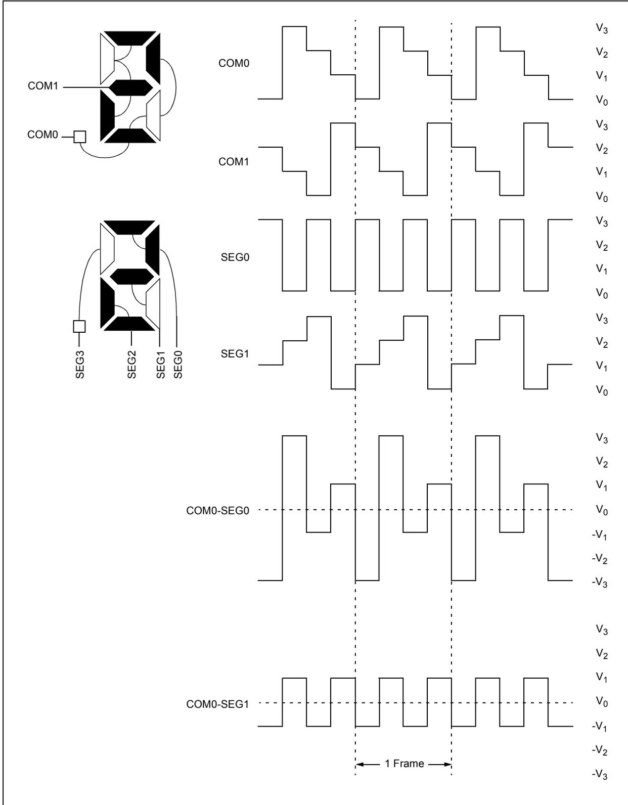
**FIGURE 22-8: TYPE-B WAVEFORMS IN 1/2 MUX, 1/3 BIAS DRIVE**
