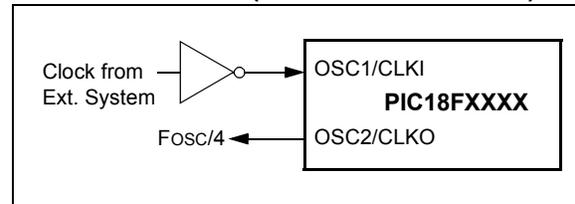
The ECIO Oscillator mode functions like the EC mode, except that the OSC2 pin becomes an additional general purpose I/O pin. The I/O pin becomes bit 6 of PORTA (RA6). Figure 2-4 shows the pin connections for the ECIO Oscillator mode.
