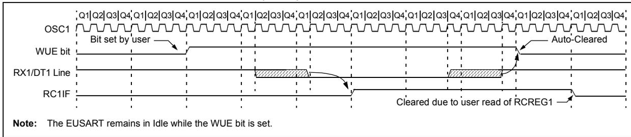
**FIGURE 16-9: AUTO-WAKE-UP BIT (WUE) TIMINGS DURING SLEEP**
