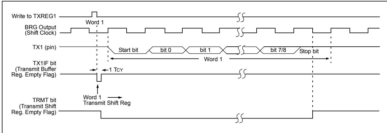
**FIGURE 16-5: ASYNCHRONOUS TRANSMISSION (BACK-TO-BACK)**
