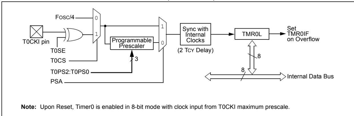
**FIGURE 10-2: TIMER0 BLOCK DIAGRAM (16-BIT MODE)**
