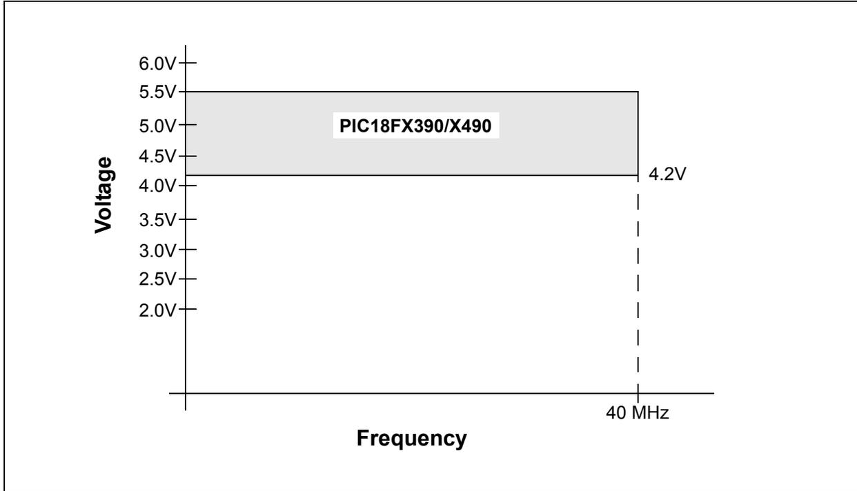
FIGURE 26-2: PIC18LF6390/6490/8390/8490 VOLTAGE-FREQUENCY GRAPH (INDUSTRIAL)
