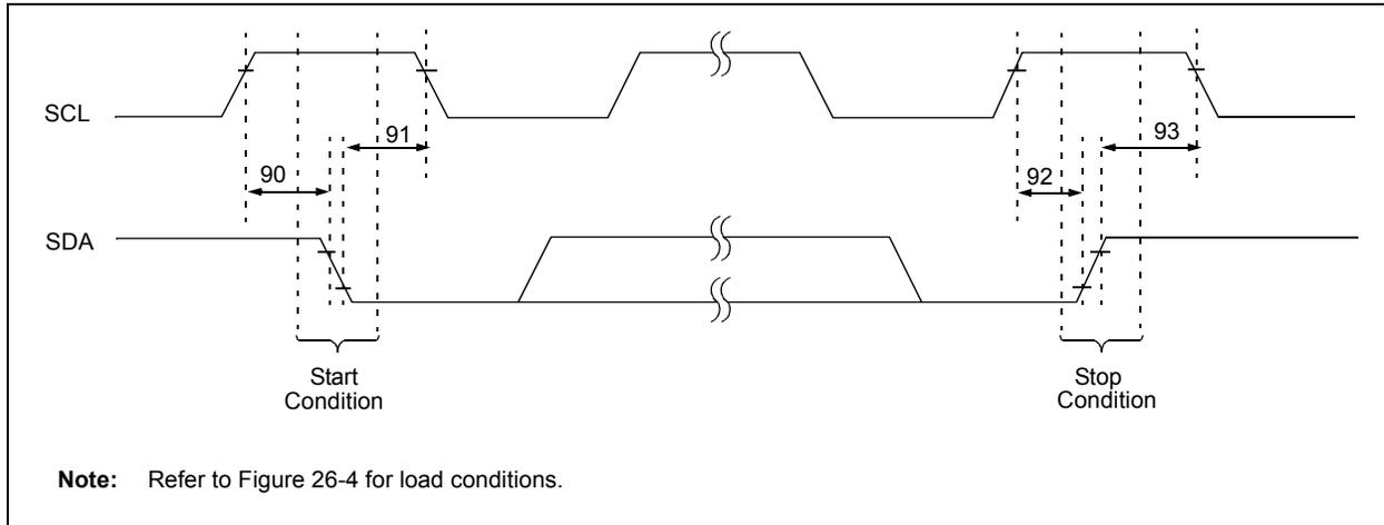
**TABLE 26-19: MASTER SSP I<sup>2</sup>C™ BUS START/STOP BITS REQUIREMENTS**
