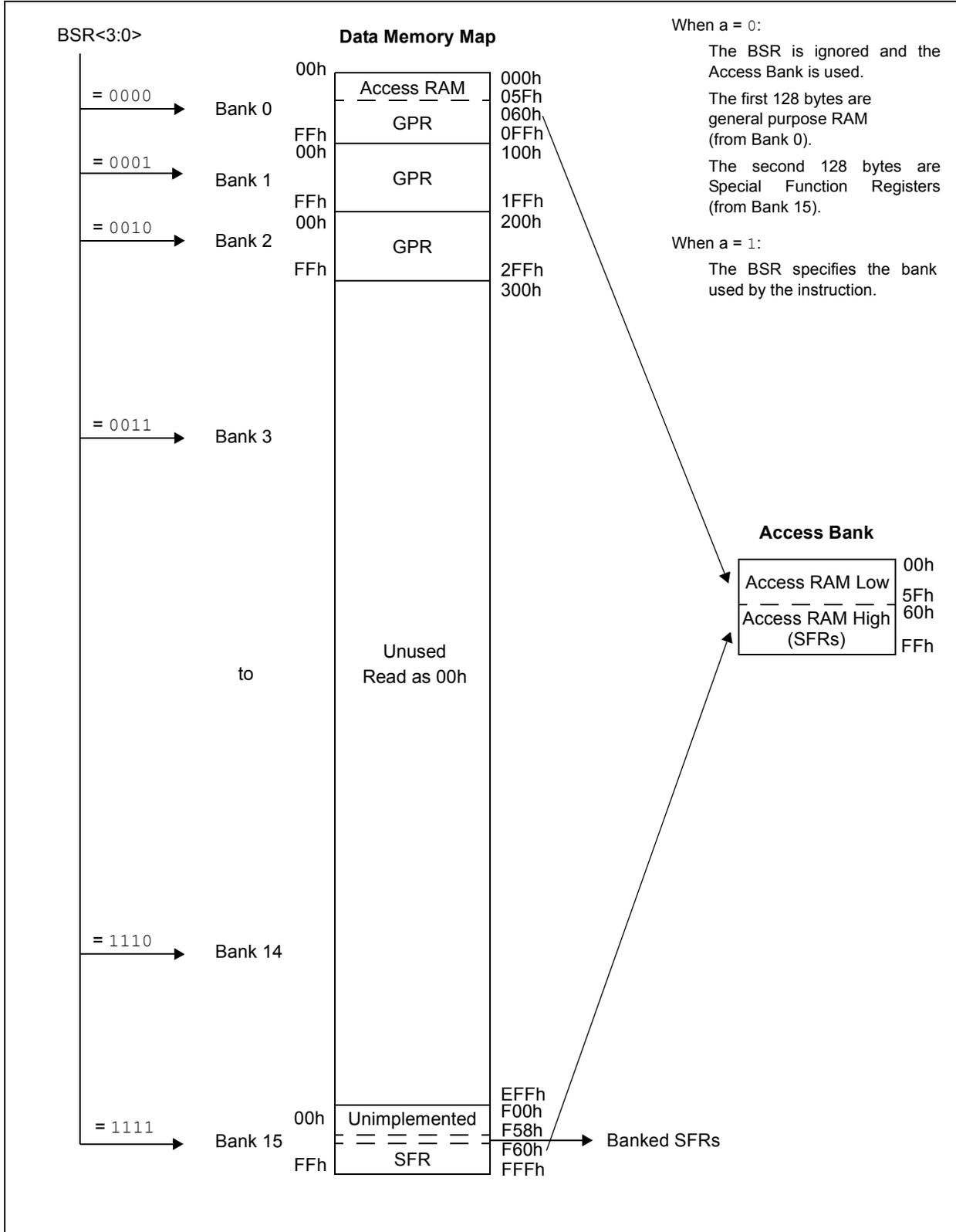
**FIGURE 5-6: USE OF THE BANK SELECT REGISTER (DIRECT ADDRESSING)**
