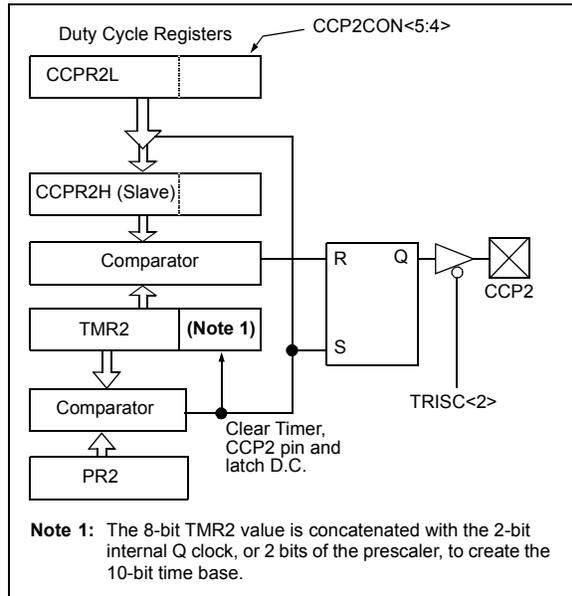
A PWM output (Figure 14-5) has a time base (period) and a time that the output stays high (duty cycle). The frequency of the PWM is the inverse of the period (1/period).
