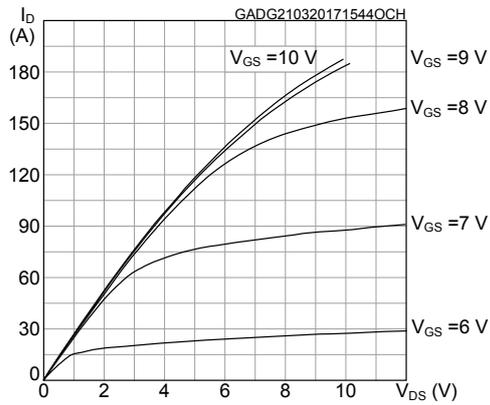
Figure 4. Transfer characteristics
