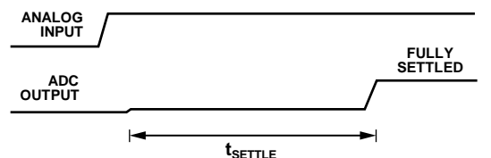
Figure 57. Step Input with Single Cycle Settling
