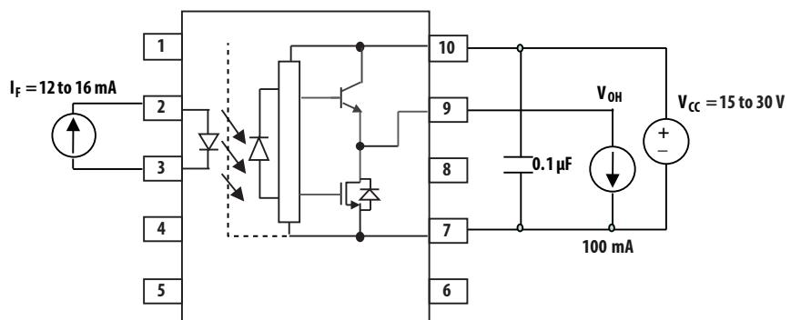
Figure 18.  $V_{OH}$  test circuit
