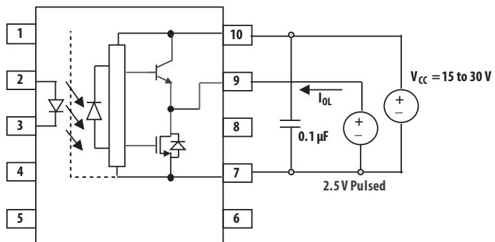
Figure 17.  $I_{OL}$  test circuit
