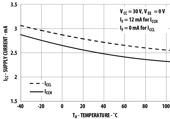
Figure 7.  $I_{CC}$  vs. temperature
