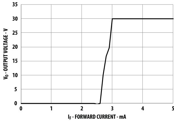
Figure 15. Transfer Characteristics
