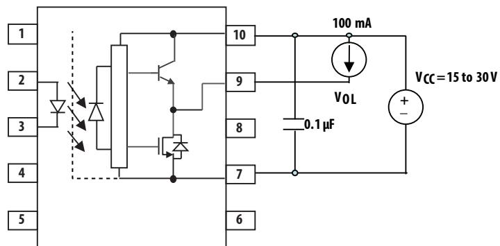
Figure 19.  $V_{0L}$  test circuit
