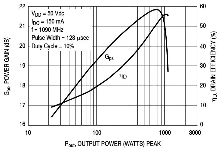
Figure 15. Power Gain and Drain Efficiency
