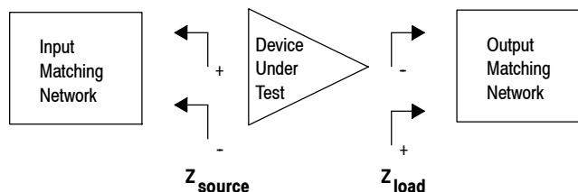
Figure 16. Series Equivalent Source and Load Impedance — 1090 MHz
