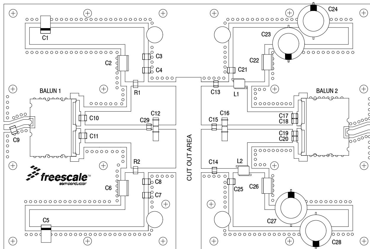
**Figure 14. MMRF1007HR5(HSR5) Test Circuit Component Layout — 1090 MHz**
