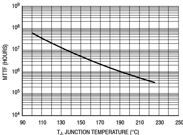
This above graph displays calculated MTTF in hours when the device is operated at  $V_{\text{DD}} = 50 \text{ Vdc}$ ,  $P_{\text{out}} = 1000 \text{ W Peak}$ , Pulse Width = 128  $\mu\text{sec}$ , Duty Cycle = 10%, and  $\eta_D = 56\%$ .
