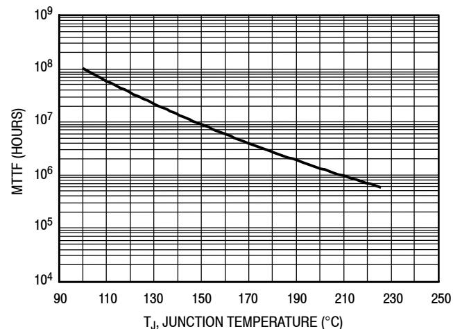
This above graph displays calculated MTTF in hours when the device is operated at  $V_{\text{DD}} = 50 \text{ Vdc}$ ,  $P_{\text{out}} = 1000 \text{ W Peak}$ , Mode-S Pulse Train, Pulse Width = 32  $\mu\text{sec}$ , Duty Cycle = 6.4%, and  $\eta_D = 59\%$ .
