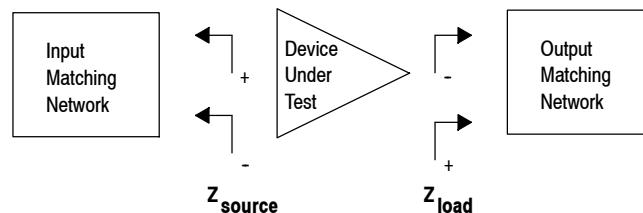
Figure 13. Series Equivalent Source and Load Impedance
