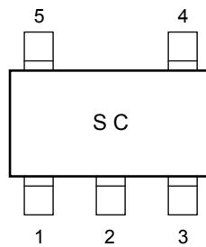
**Pin Connection (top view)**
