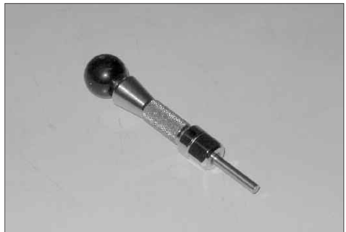
Extraction tool for contact # 8: 51 06 021 0936 Extraction tool tip: 51 06 021 3436
