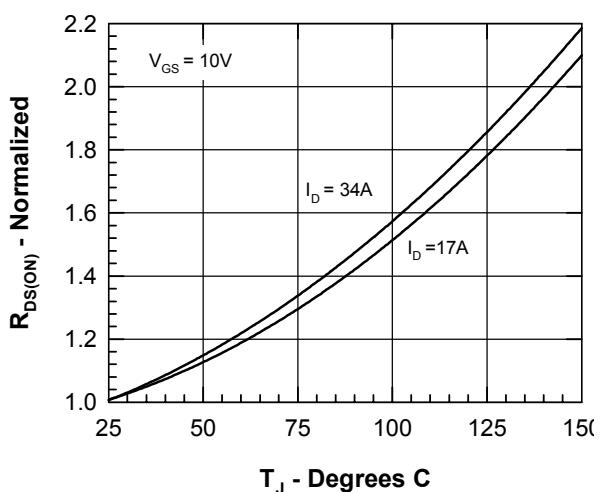
Figure 4.  $R_{DS(on)}$  normalized to  $0.5 I_{D25}$  value vs.  $T_J$
