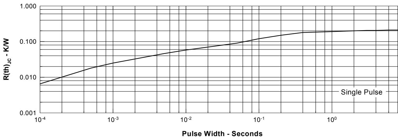
Figure 9. Transient Thermal Resistance
