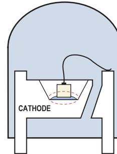
Note: Electrical connection between bottom surface of LED die and the lead frame is achieved through conductive paste.
