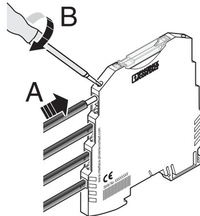
Figure 4 Screw connection
