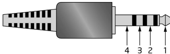
Figure 4. 4-Pin 3.5 mm (1/8 inch) Audio Jack Pin Out
