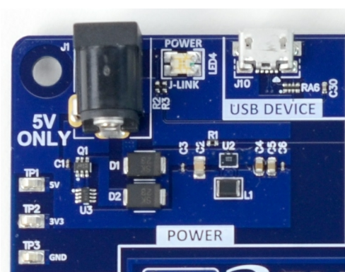
Figure 4: Power Section of Main Board
