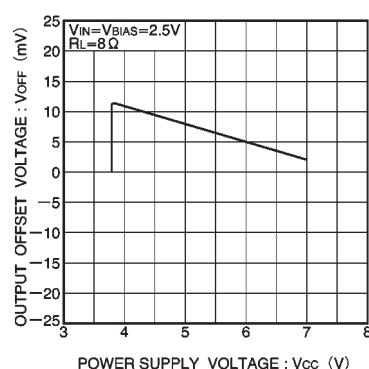
Fig.6 Power supply voltage vs. output offset voltage
