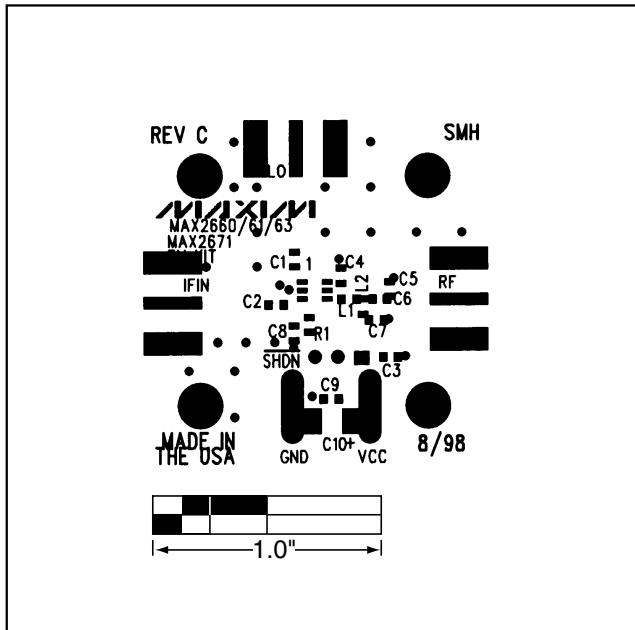
Figure 2. MAX2660 EV Kit PC Board Layout—Component Side
