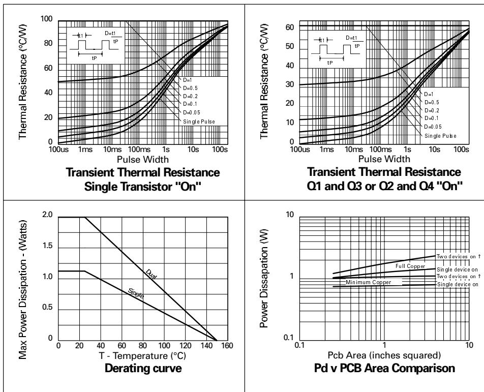
\* The power which can be dissipated assuming the device is mounted in a typical manner on a PCB with copper equal to 2 inches square.
