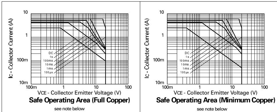
Note: The Safe Operating Area (SOA) charts shown are a combination of the worst case secondary breakdown characteristics for the NPN/PNP pair, and the thermal curves demonstrating the power dissipation capability of the energised ZHB part (opposing NPN-PNP switched on) when mounted on a 50mm x 50mm FR4 PCB. The two cases show:
