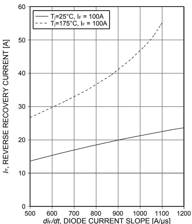
Figure 24. Typical reverse recovery current as a function of diode current slope
