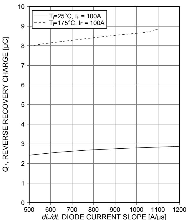
Figure 23. Typical reverse recovery charge as a function of diode current slope
