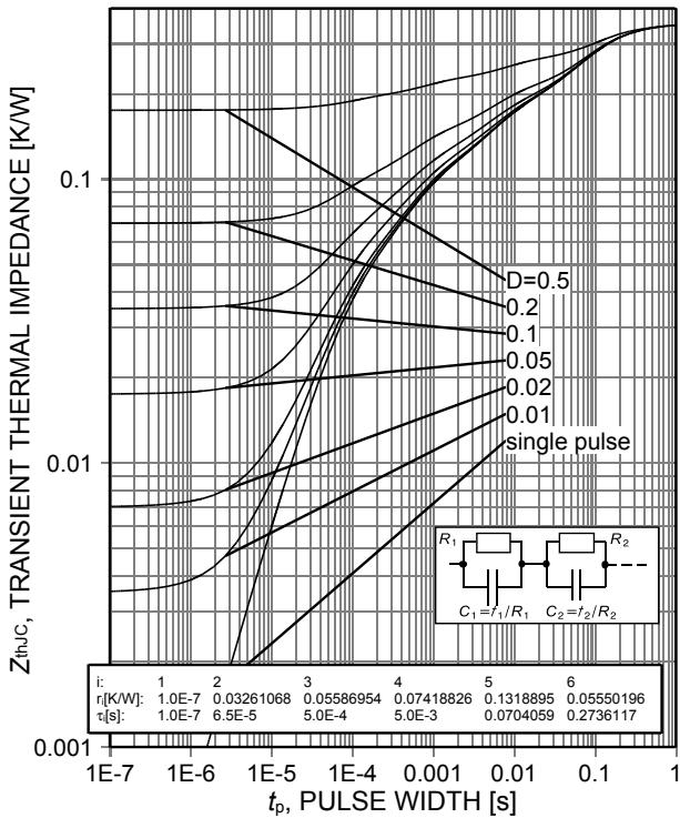
Figure 21. Diode transient thermal impedance as a function of pulse width for different duty cycles  $D$
