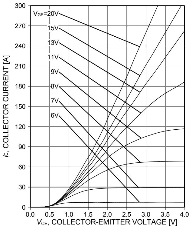
**Figure 5. Typical output characteristic**
