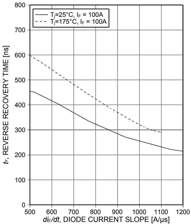
Figure 22. Typical reverse recovery time as a function of diode current slope
