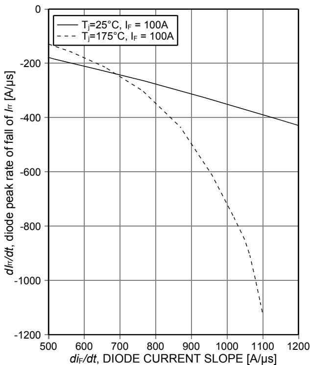
Figure 25. Typical diode peak rate of fall of reverse recovery current as a function of diode current slope
