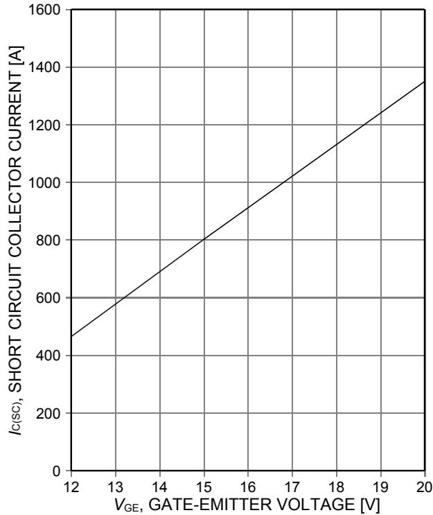
**Figure 18. Typical short circuit collector current as a function of gate-emitter voltage**
