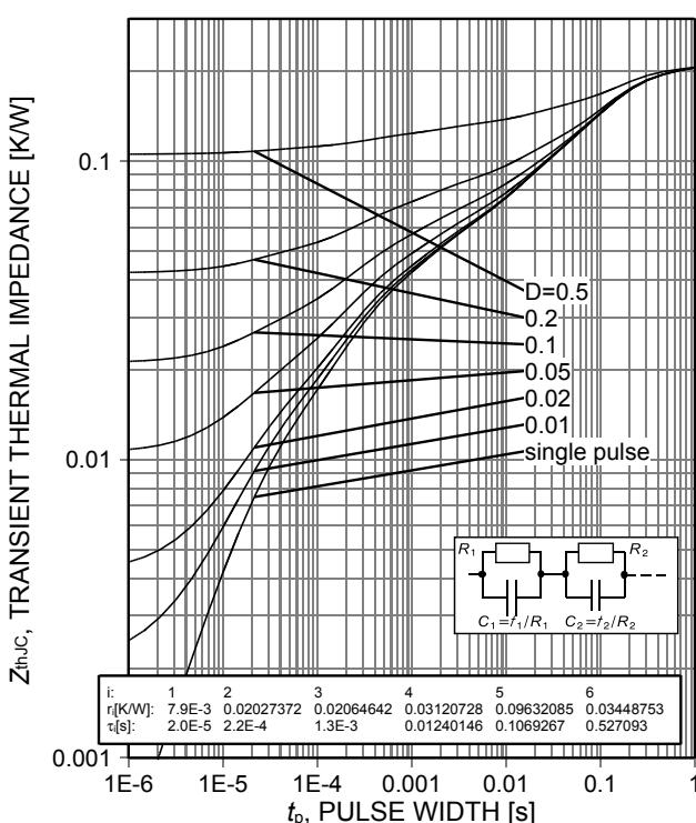
**Figure 20. IGBT transient thermal impedance as a function of pulse width for different duty cycles  $D$**
