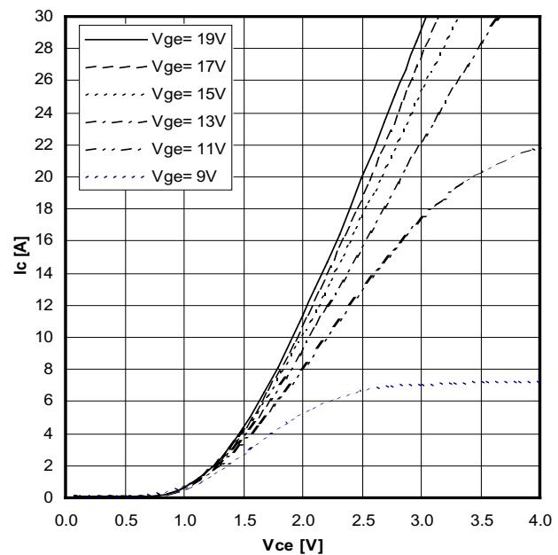
Typical output characteristics ( $125\text{ }^\circ\text{C}$ )
