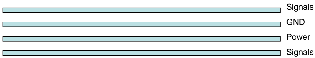
Figure 10: Typical 4-layer PCB construction
