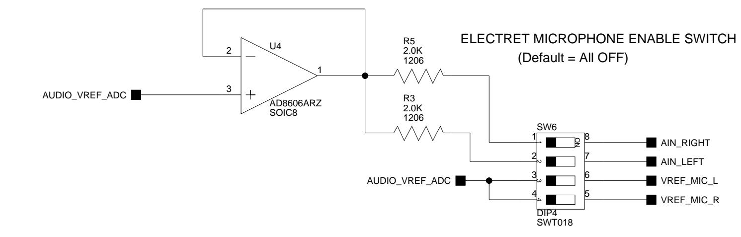
WHEN USING AN ELECTRET MICROPHONE
