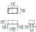
Terminal thickness = 0.15.006General tolerance:  $\pm 0.1 \pm .004$
