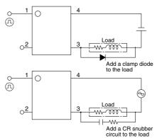
2) Even if spike voltages generated at the load are limited with a clamp diode if the circuit wires are long, spike voltages will occur by inductance. Keep wires as short as possible to minimize inductance. • Check the connection diagrams in the catalog and be sure to connect the terminals correctly.
