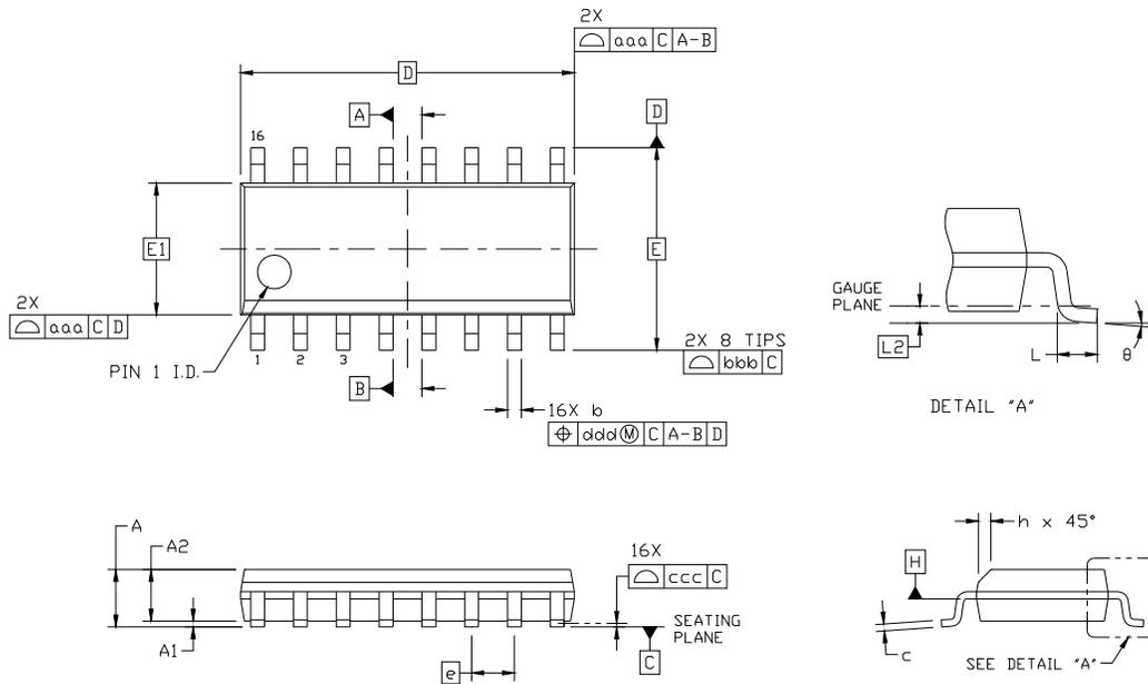
**Figure 5. 16-Pin SOIC**
