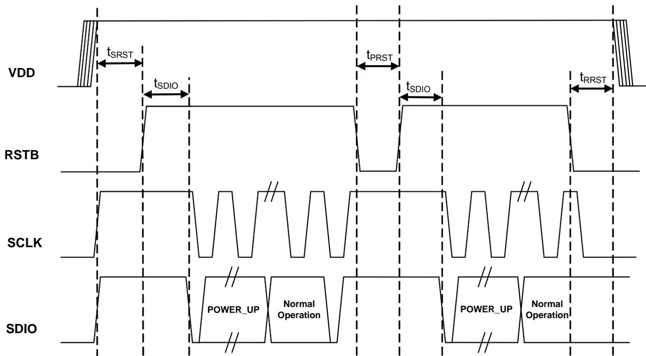
**Figure 1. Reset Timing**
