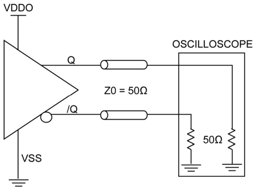
Figure 4. HCSL Output Load and Test Circuit
