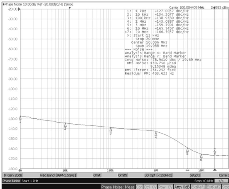
Phase Noise Plot: 100MHz, 12kHz – 20MHz 254fS
