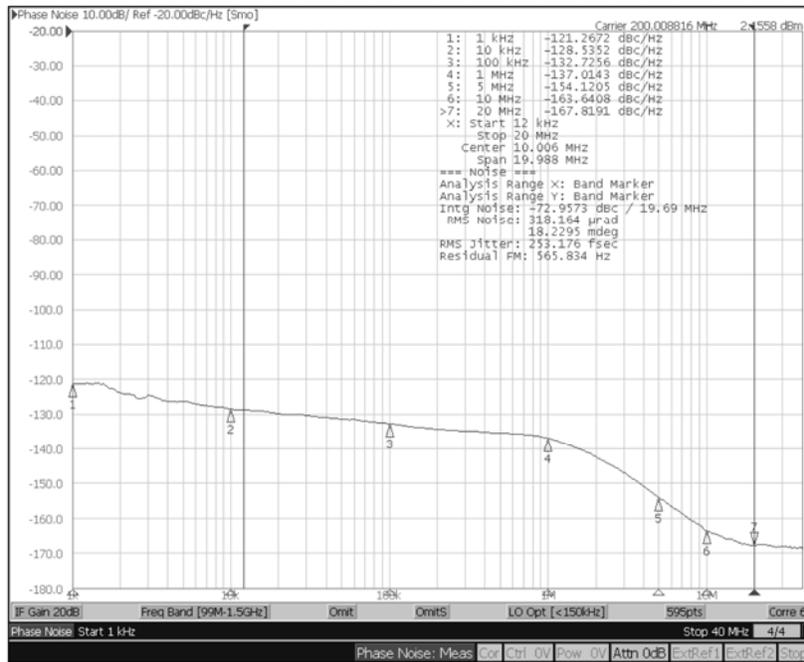
Phase Noise Plot: 200MHz, 12kHz – 20MHz 253fS
