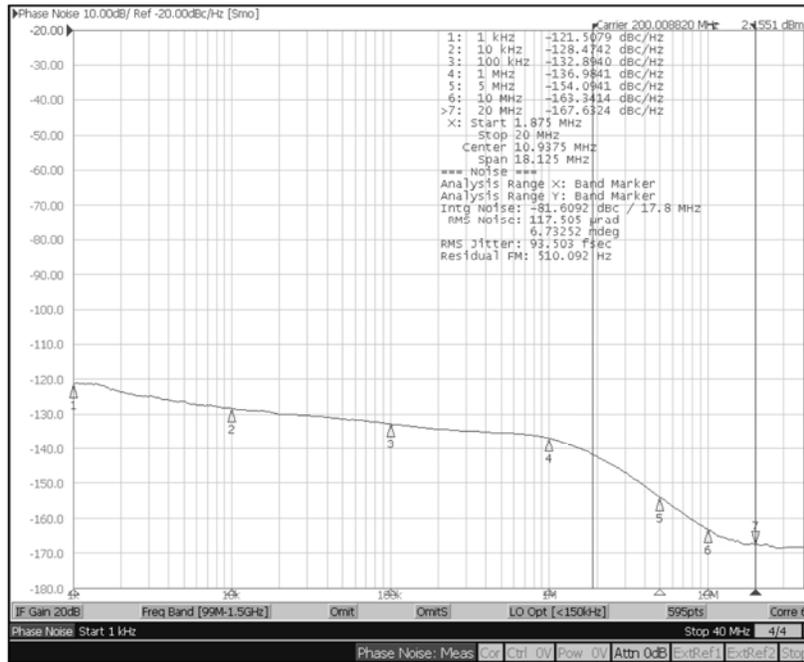
Phase Noise Plot: 200MHz, 1.875MHz – 20MHz 94fS
