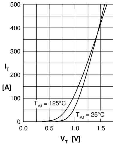
Fig. 1 Forward characteristics
