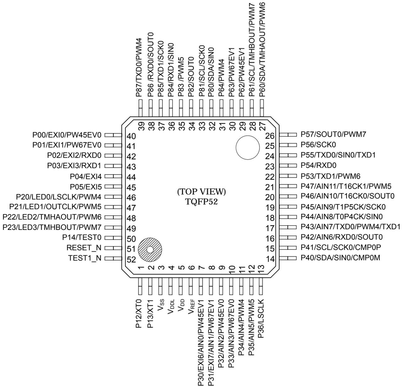
Figure 1-5 Pin Layout of ML620Q154A/ML620Q155A/ML620Q156A TQFP52 Package
