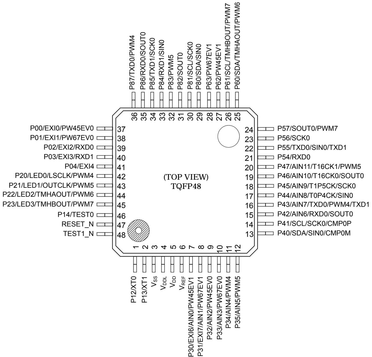
Figure 1-4 Pin Layout of ML620Q151A/ML620Q152A/ML620Q153A TQFP48 Package
