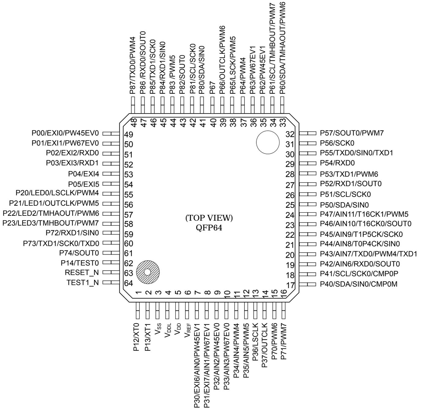
Figure 1-6 Pin Layout of ML620Q157A/ML620Q158A/ML620Q159A QFP64 Package
