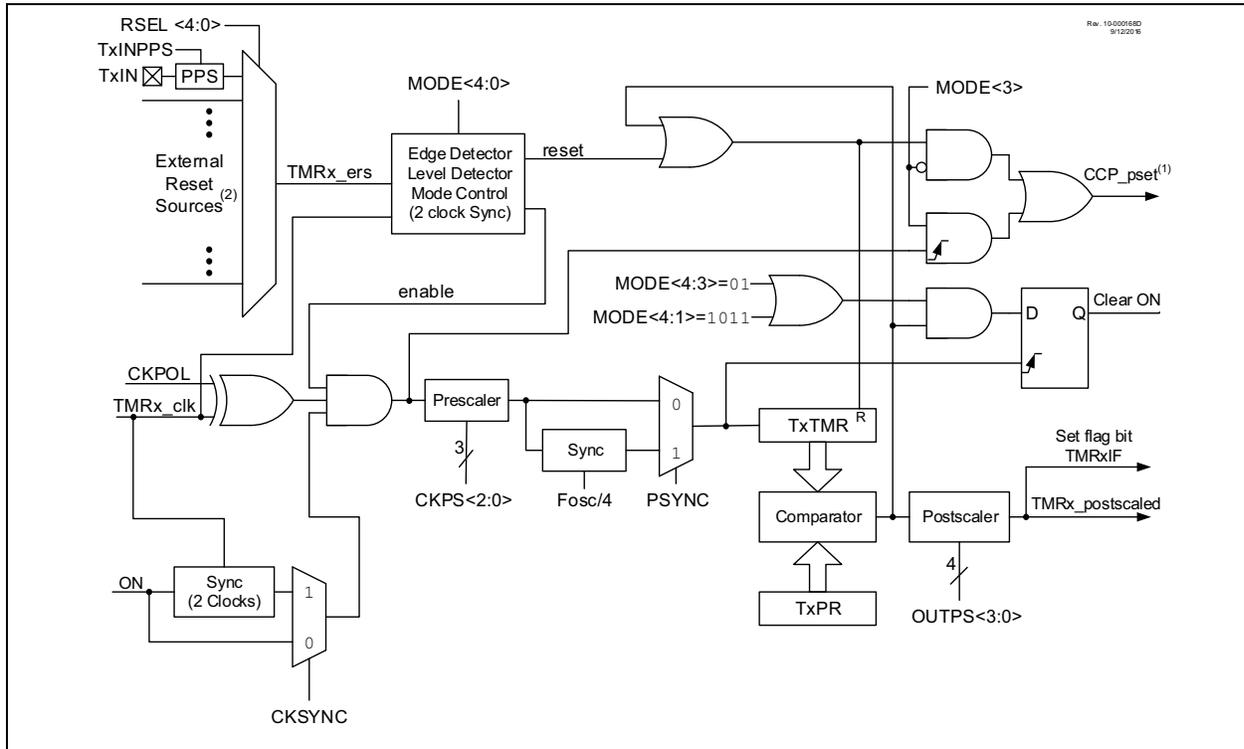
**FIGURE 22-2: TIMER2 CLOCK SOURCE BLOCK DIAGRAM**
