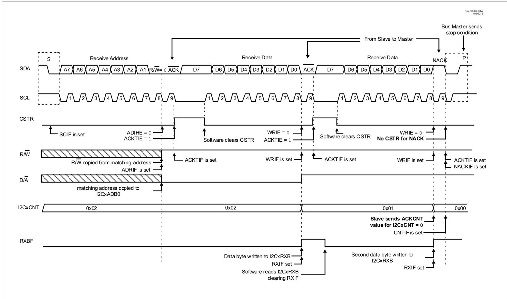
FIGURE 33-8: I<sup>2</sup>C SLAVE, 7-BIT ADDRESS, RECEPTION NO I2CxCNT (ACKTIE = 0, ADRIE = 1, WRIE = 1)
