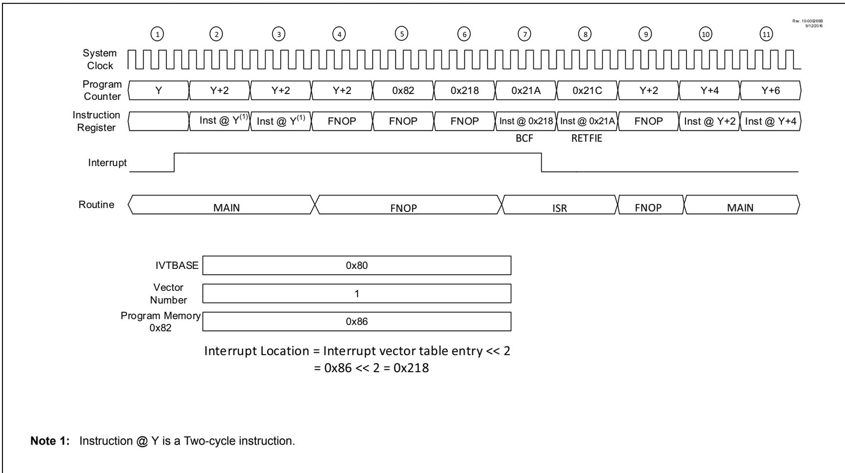
**FIGURE 9-9: INTERRUPT TIMING DIAGRAM - THREE CYCLE INSTRUCTION**
