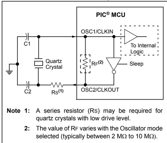
**FIGURE 7-4: CERAMIC RESONATOR OPERATION (XT OR HS MODE)**
