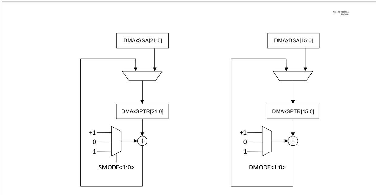
The DMA can initiate data transfers from the PFM, Data EEPROM or SFR/GPR Space. The SMR<1:0> bits in the DMAxCON1 register are used to select the type of memory being pointed to by the Source Address Pointer. The SMR<1:0> bits are required because the PFM and SFR/GPR spaces have overlapping addresses that do not allow the specified address to uniquely define the memory location to be accessed.
