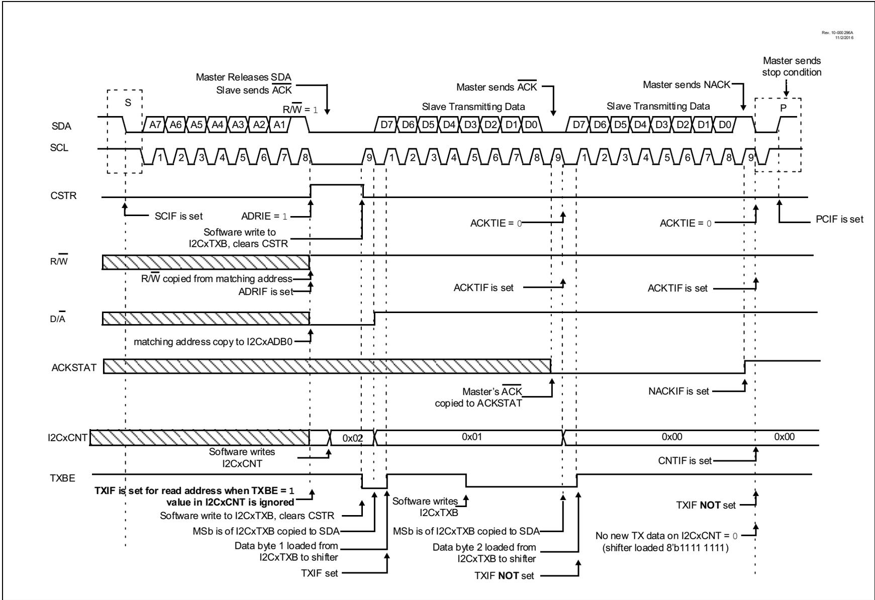
**FIGURE 33-10: I<sup>2</sup>C SLAVE, 7-BIT ADDRESS, TRANSMISSION (NO CLOCK STRETCHING)**
