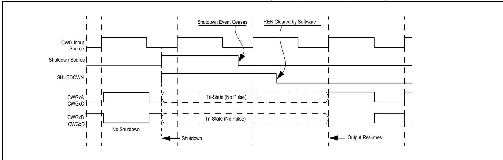
FIGURE 26-16: SHUTDOWN FUNCTIONALITY, AUTO-RESTART ENABLED (REN = 1, LSAC = 01, LSBD = 01)
