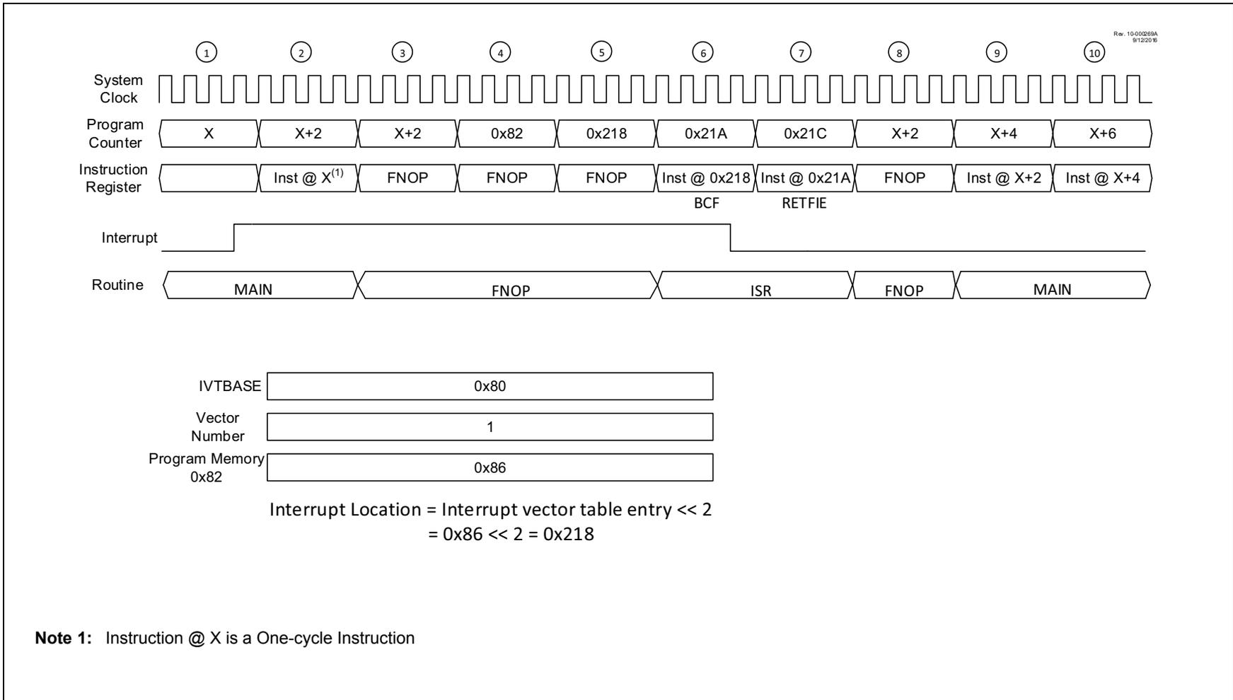
**FIGURE 9-8: INTERRUPT TIMING DIAGRAM - TWO WORD INSTRUCTION**
