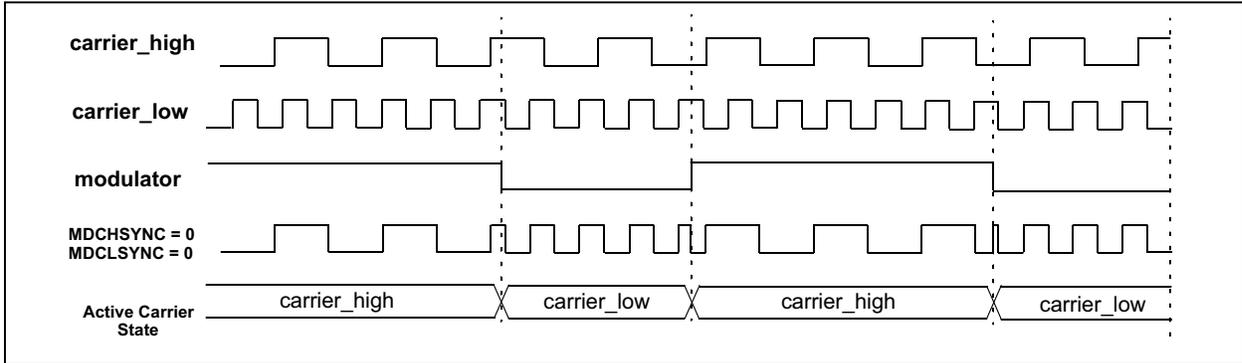
**FIGURE 30-4: Carrier High Synchronization (CHSYNC = 1, CLSYNC = 0)**
