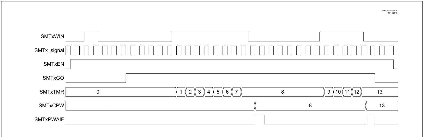
**FIGURE 25-20: GATED COUNTER MODE SINGLE ACQUISITION TIMING DIAGRAM**
