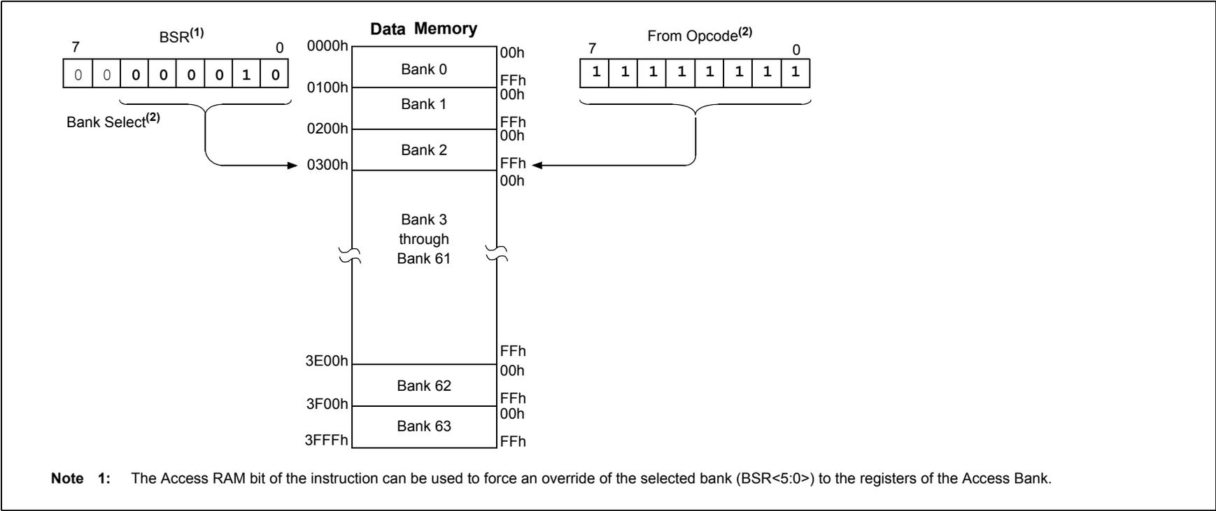
**Note 1:** The Access RAM bit of the instruction can be used to force an override of the selected bank (BSR<5:0>) to the registers of the Access Bank.
