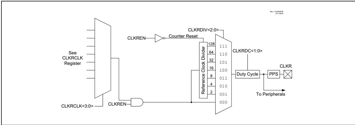
**FIGURE 8-2: CLOCK REFERENCE TIMING**
