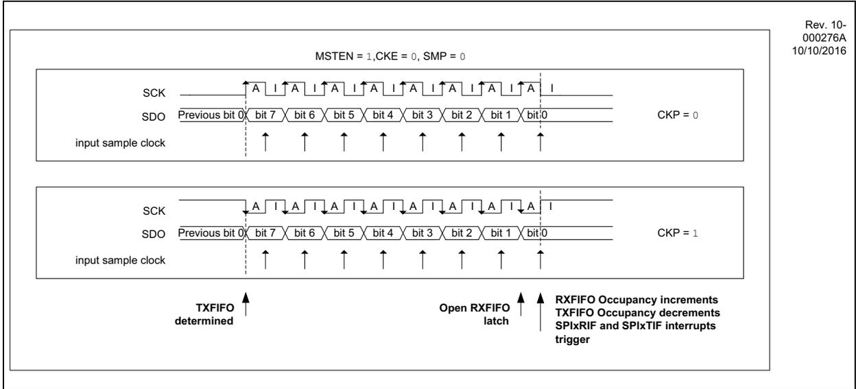
**FIGURE 32-8: CLOCKING DETAIL - MASTER MODE, CKE/SMP = 1/1**
