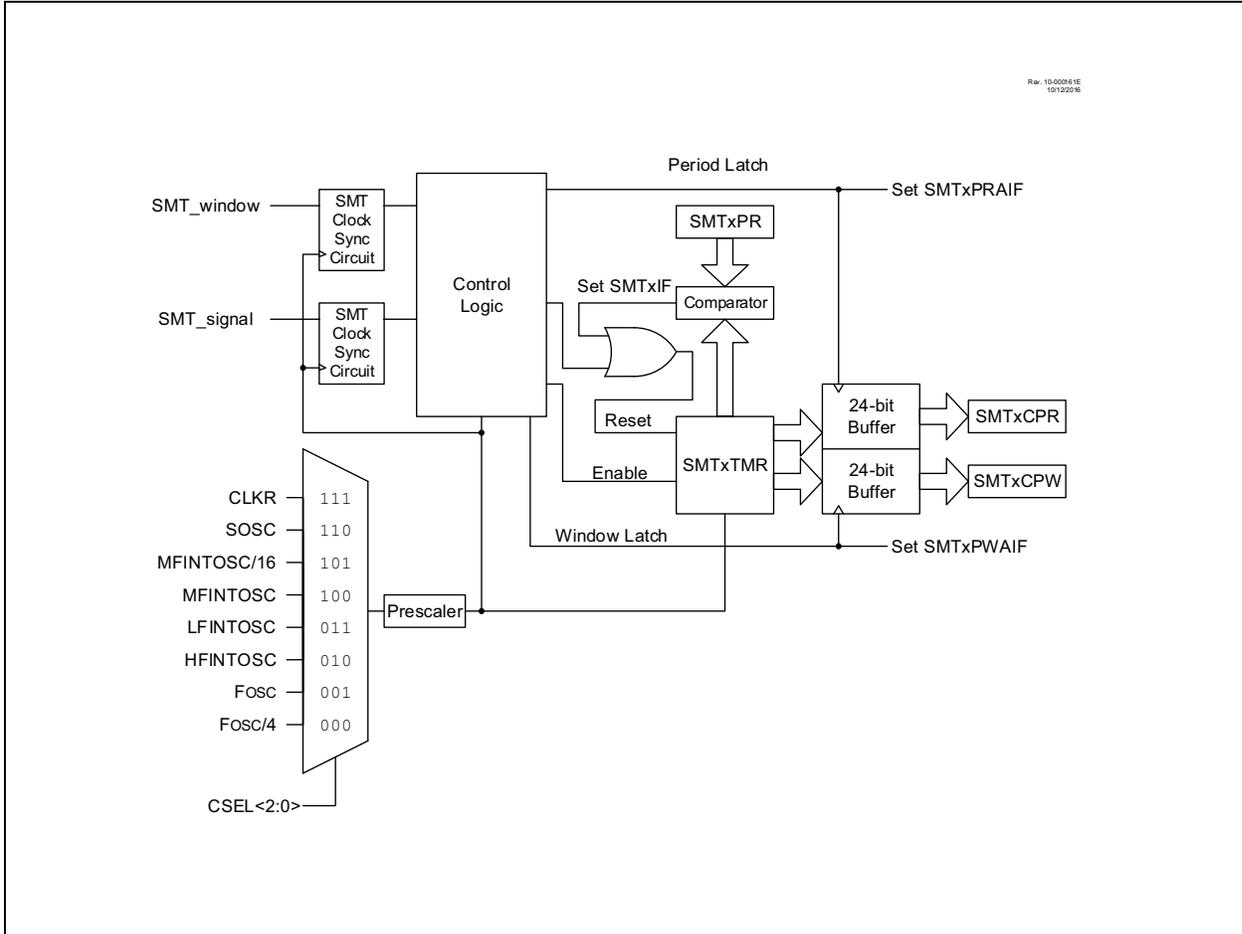
**FIGURE 25-2: SMT SIGNAL AND WINDOW BLOCK DIAGRAM**
