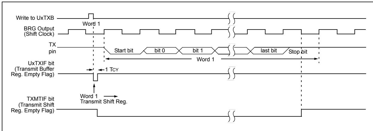
**FIGURE 31-4: ASYNCHRONOUS TRANSMISSION (BACK-TO-BACK)**
