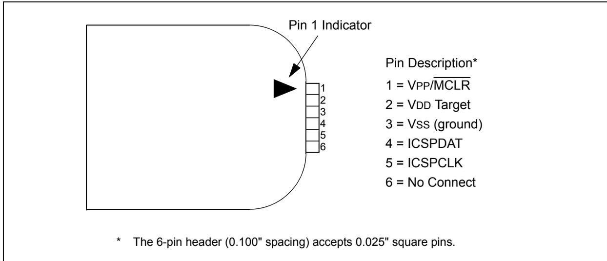
**FIGURE 40-3: TYPICAL CONNECTION FOR ICSP™ PROGRAMMING**
