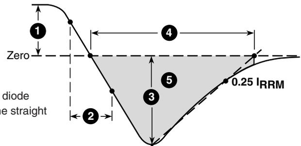
Figure 10, Diode Reverse Recovery Waveform and Definitions
