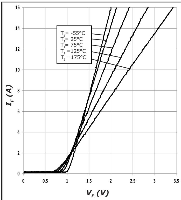
Figure 1. Forward Characteristics
