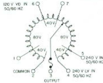
For opposite rotation interchange external connections from 5 to 1, 2 to 4 and 6 to 7.
