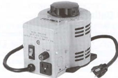
**L SERIES:** A selected grouping of variable transformers packaged in a deluxe aluminum enclosure, three-conductor line cord, plug, matching receptacle, pilot light, switch and fuse. An ammeter and voltmeter are available on the 10 amp model.
