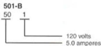
2. In a 4 digit number where the third digit is 1, the first two digits indicate amperes, the third designates 120 volts.
