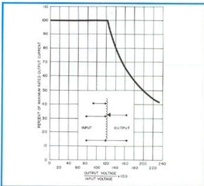
Figure B. Max Output Current — Dual Voltage
