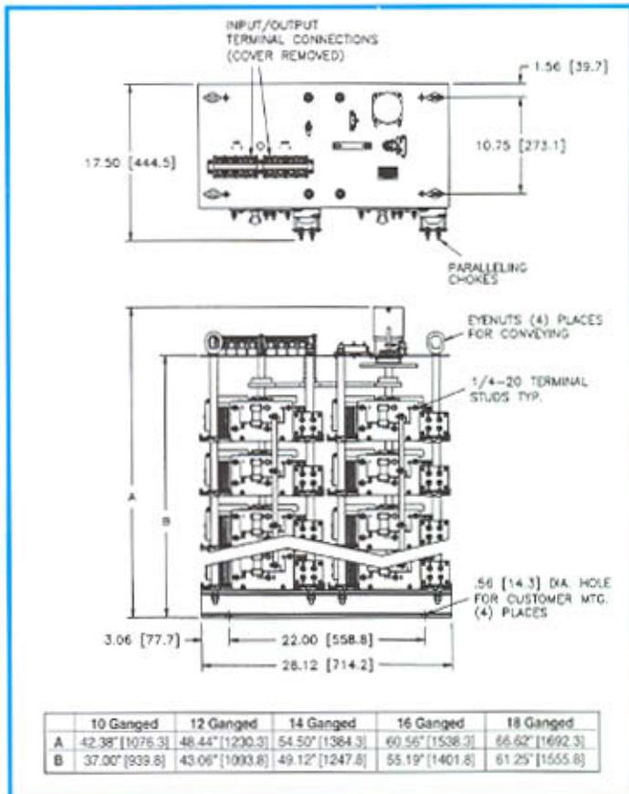
Motor-Driven 10, 12, 14, 16 & 18-Ganged Open Delta & Parallel, Uncased
