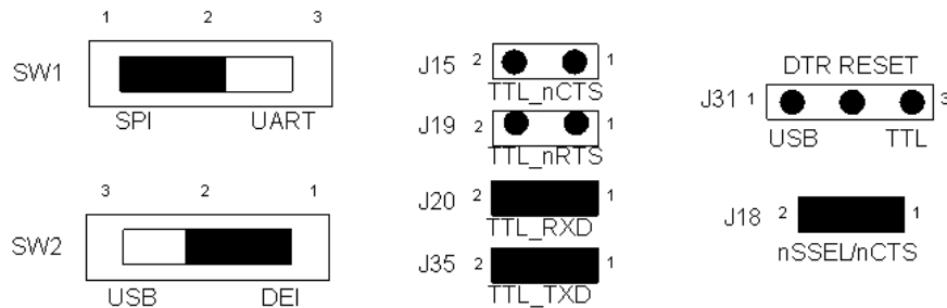
Figure 6. Jumper settings required for on-board host microcontroller UART access by InSight Adapter
