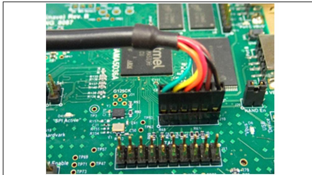
3. On the PC, open a serial port session using TeraTerm, PuTTY or similar communication software. The settings are 115200 baud, 8 bits, no parity, 1 Stop bit (8N1).
