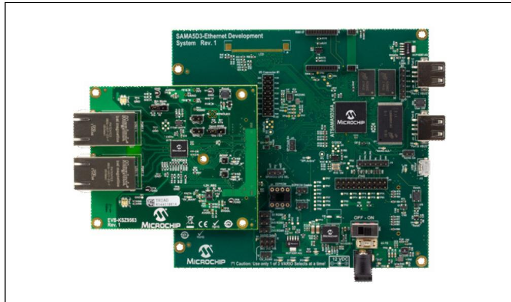
5. Connect a 12V power adapter to the SAMA5D3 EDS board. When the board is powered on, it boots the installed Linux operating system.
