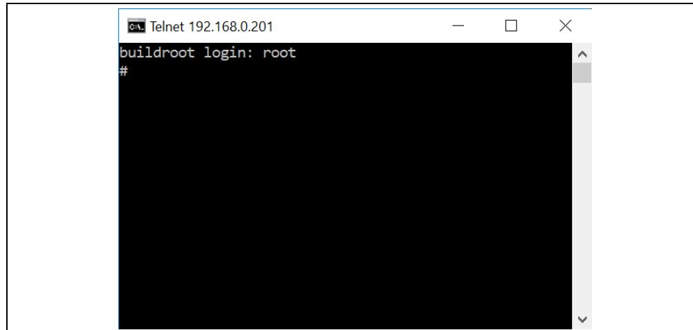
7. The Linux file system root is located with command: cd /
