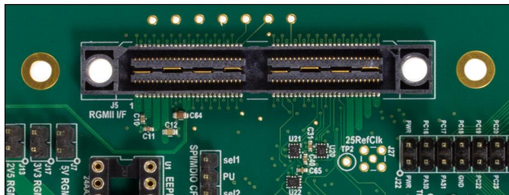
A daughter board receives power from the SAMA5D3 EDS board via any of the available supplies: VDDIOP1 (VARIO), 2V5, 3V3, 5V, or 12V. The daughter board documentation specifies which power rail(s) are used. Jumpers J3, J7, J13, and J17 are used to connect/disconnect 12V, 5V, 3V3, and 2V5 to this connector. Normally, all of these jumpers should be installed even if some voltages are not needed by the daughter board.
