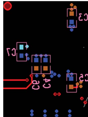
Figure 61. Bottom Layer Decoupling
