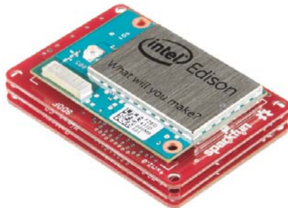
9 DOF Block Installed
