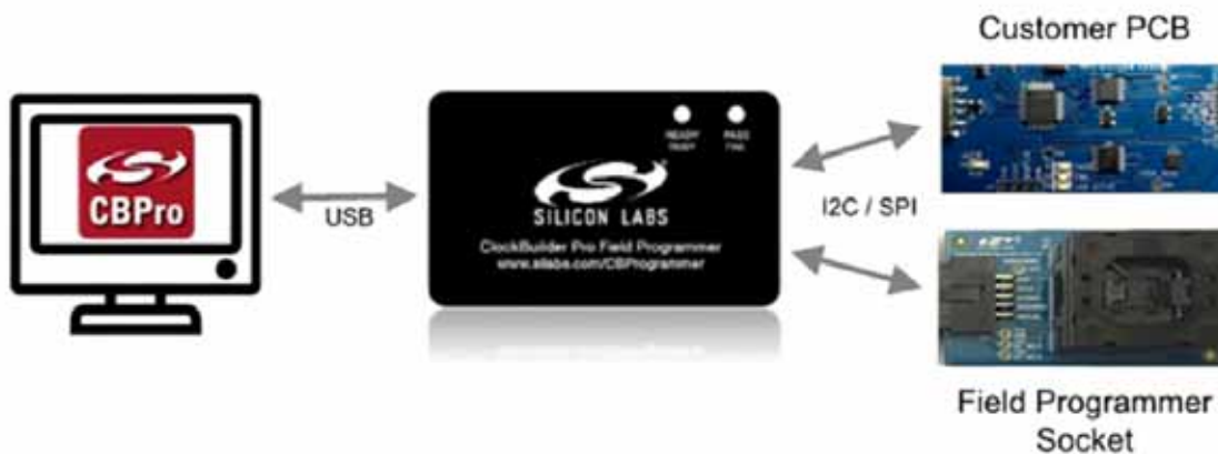
Figure 5. PC to CBPROG-DONGLE Connection
