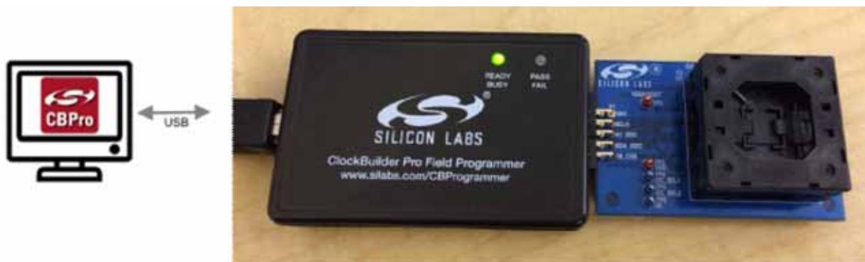
Figure 7. System from PC to Programming CBPROG-DONGLE Board to QFN Field Programmer Socket Board
